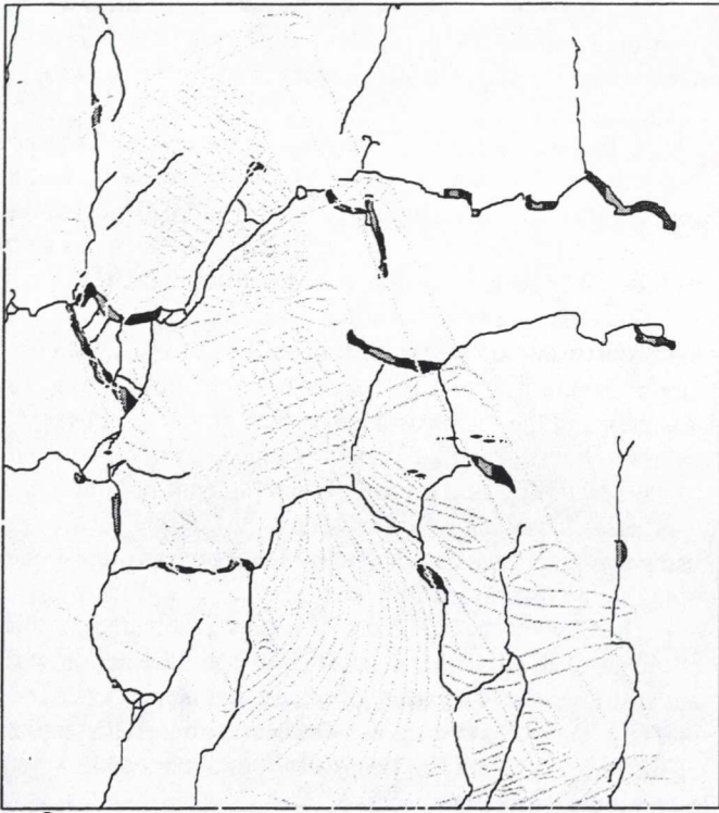
Figure 37.6: Recording of fissures and missing parts by the computer system.
