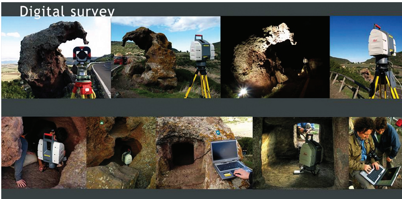
Fig. 9. Working at the Rock survey: two days, ten scanner positions, a specific topographical network, twenty five millions of points gathered with a coverage of the ninety-five percent of the outer and inner surface.
