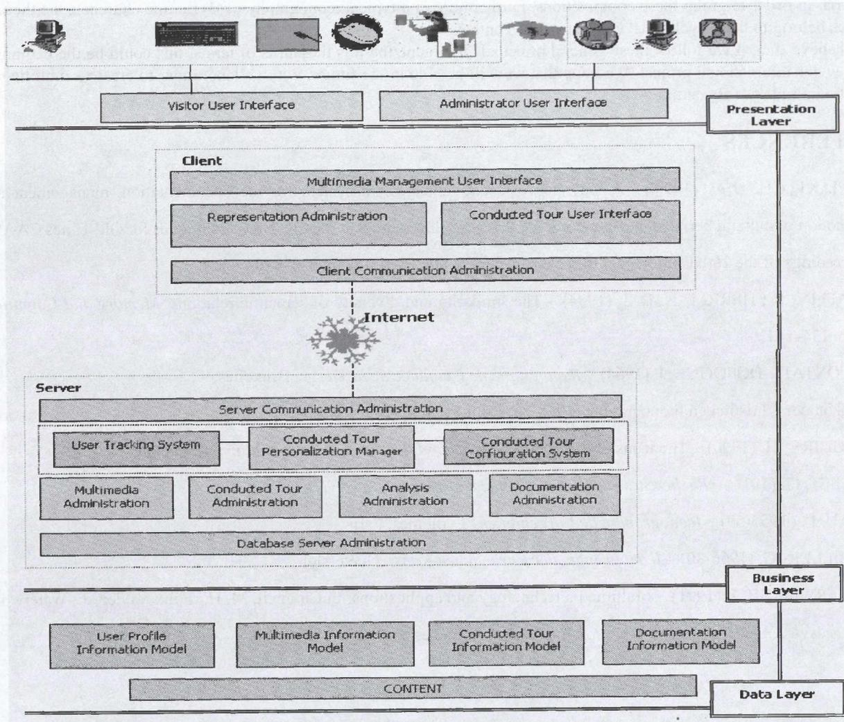
Fig. 1 – System Architecture.
