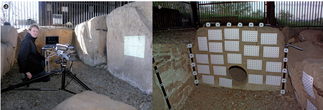
Fig. 3. a) The measurement system in front of a wall stone with illuminated measurement field. b) The port-hole slab with attached control points.
