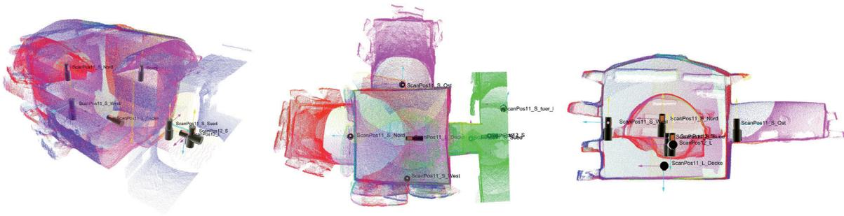
Fig. 1. Point cloud cluster of cubiculum with inserted scanner symbols, perspective view, top view and side view.
