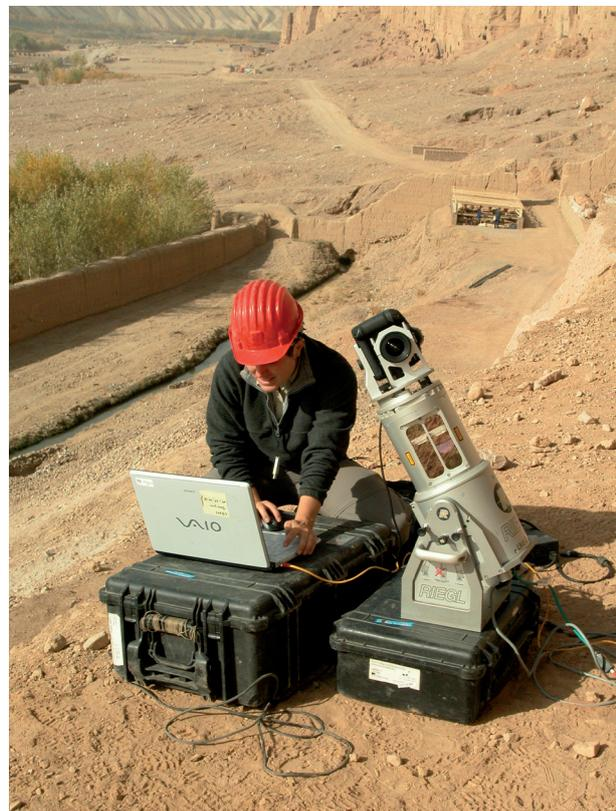
Fig. 4. Laser Scanner LMS 420i.
