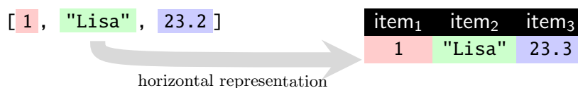
Figure 2.12: Horizontal representation of an array in a database. Order is implicitly given by the position of the columns.
