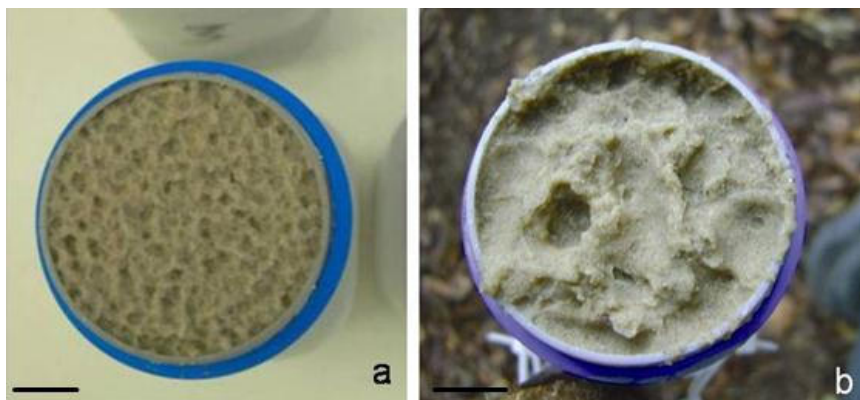
Fig. 4: Sand detachment from splash cups under open field (a) and under forest vegetation (b) (black line = 1 cm).
