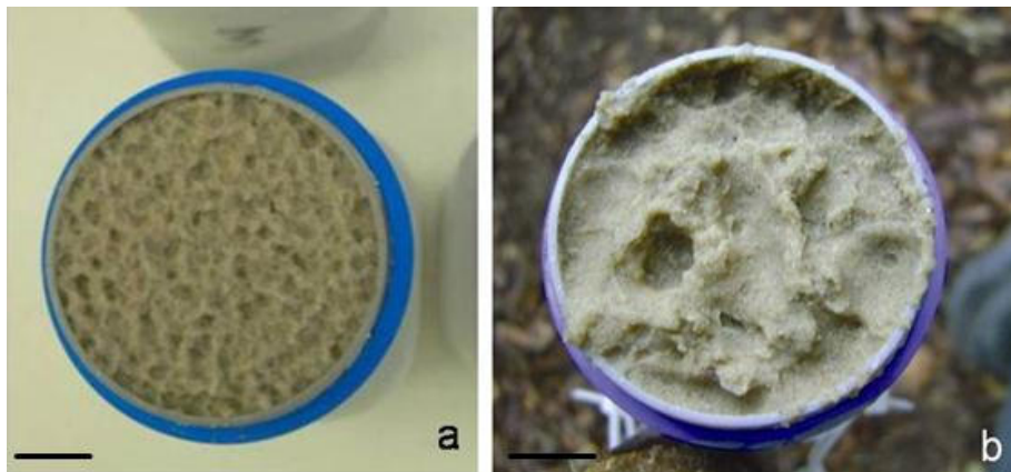
Fig. 9: Sand detachment from splash cups under open field (a) and under forest vegetation (b) (black line = 1 cm).
