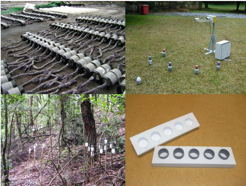
Fig. 2: Disassembled splash cups (upper left), styrofoam cup carrier for the field (upper right), setup for the calibration measurements with splash cups and laser disdrometer (lower left), and setup of splash cups and throughfall collectors under forest vegetation (lower right).
