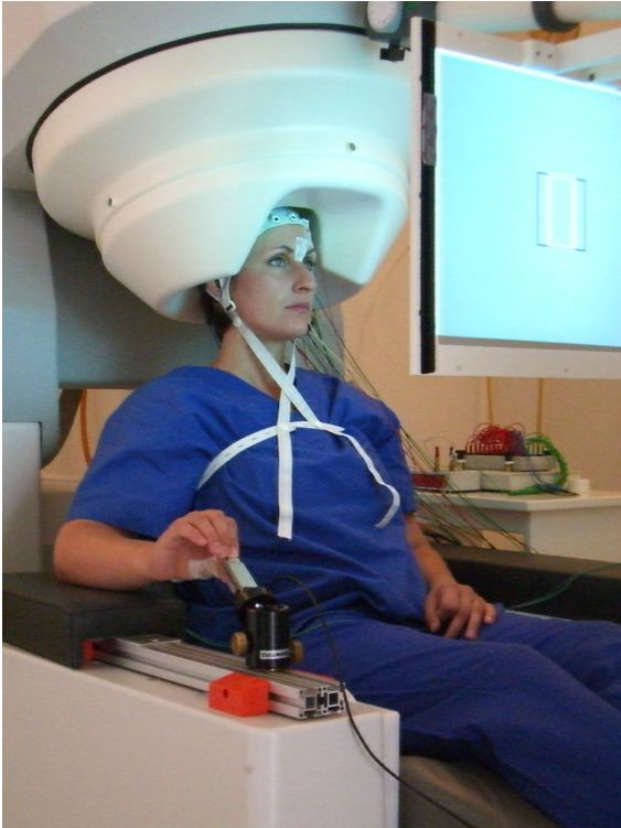
Figure 2.1: Experimental Setup of the study on visuomotor integration. Inside a magnetically shielded room, subjects were placed with their head carrying the EEG cap in a helmet shaped dewar. The screen displaying the feedback and the fixation cross was \sim 1 m in front of the subject and the pinch grip to the subject's right side.
