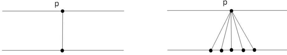
Fig. 4.5: If the PWCC holds, position p can be part of at most one edge to each other sequence (left). Generally however there can be arbitrary many edges from p to each other sequence. The maximum possible number of such edges is called the maximum pairwise segment spread (MPSS) and in this example (right) it is bounded by 5.
