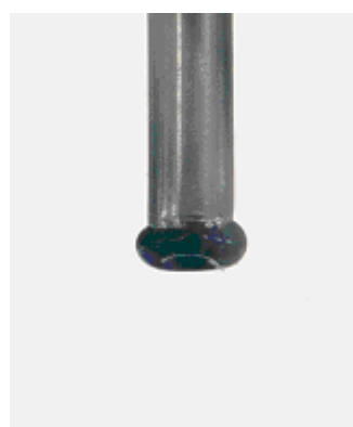
Figure 3.2b Retraction of coal tar without apparent aging (9 days)
