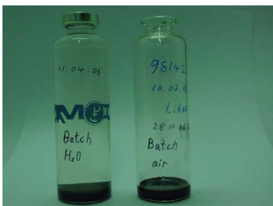
Figure 3.8 Setting up of the batch experiments coal tar open to water and air
