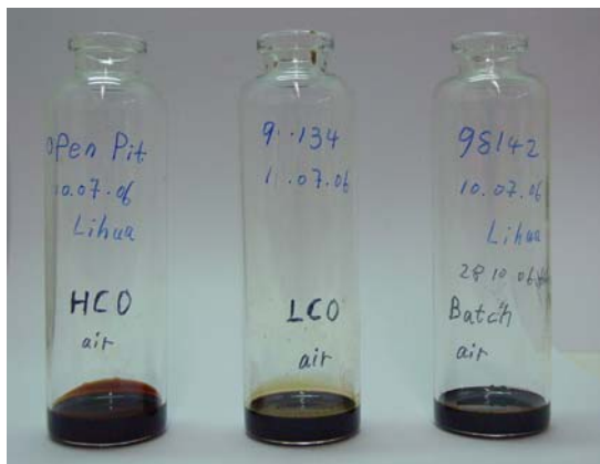
Figure 3.9 Setting up of batch experiments heavy and light crude oil open to air
