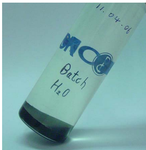
Figure 3.12 Batch experiment of coal tar, free-flowing NAPL inside a full of water vial
