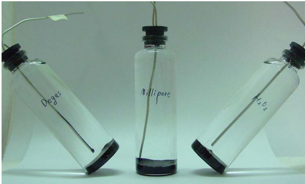
Figure 3.13 Results of CWFTE, all of them showed solid or semi-solid interfacial phase
