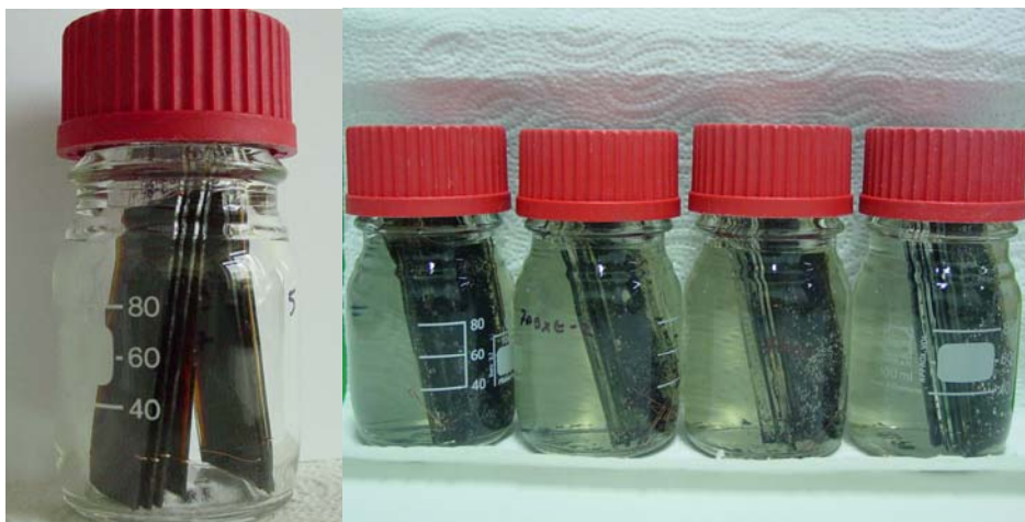
Figure 4.1. Batch experiment performed with the aged coal tars coating on the surface of the glass plates.
