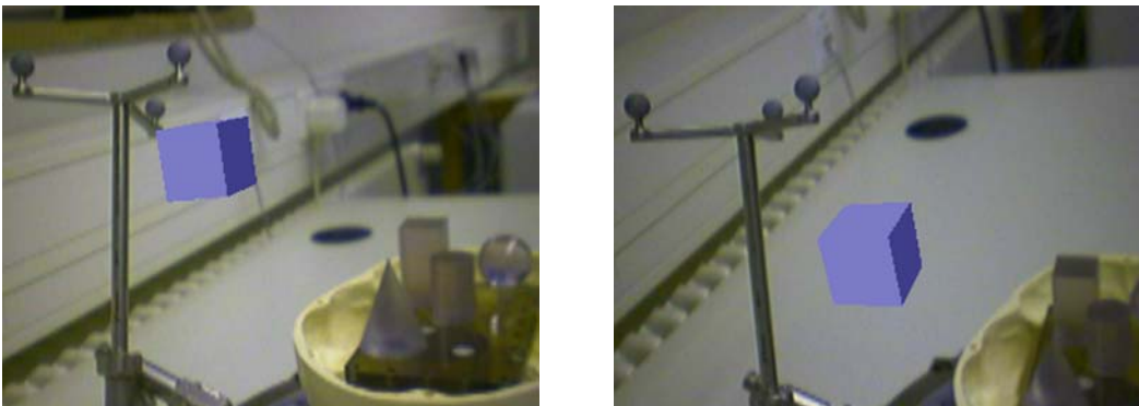
Figure 2.13: Early overlay experiments with ARGUS . The blue cube is a virtual object. It is displayed with a correct position and orientation relative to the reference star (seen at left) based on the current camera position.
