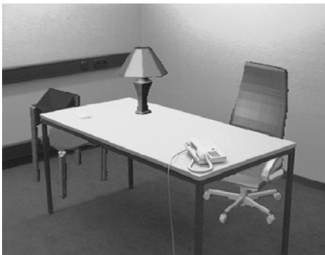
(a) Static occlusion handling with phantom models. In this image, the chairs and lamp are virtual models. The virtual chairs are correctly occluded by the real table (from [64]).
