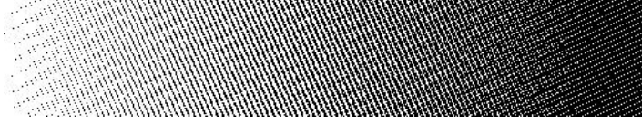
Figure 4.8: Black-and-white pattern generated by the halftoning method for the continuous intensity range [0; 1] .
