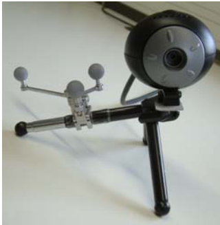
Figure 3: Webcam with attached marker clamp.
