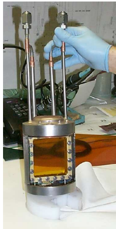
Figure 2.10: Photograph of target cell: shown is the inner target cell without the two outer cylindrical windows.
