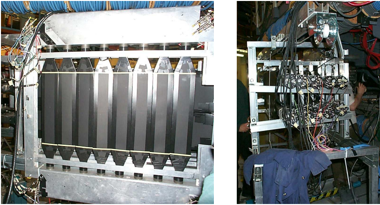
Figure 2.9: Photographs of the range telescope: the front view shows the first layer which is segmented into 8 vertical paddles, the side view shows the 6 layers and the photomultiplier tubes attached to each of the two bars of layers 2 to 6
