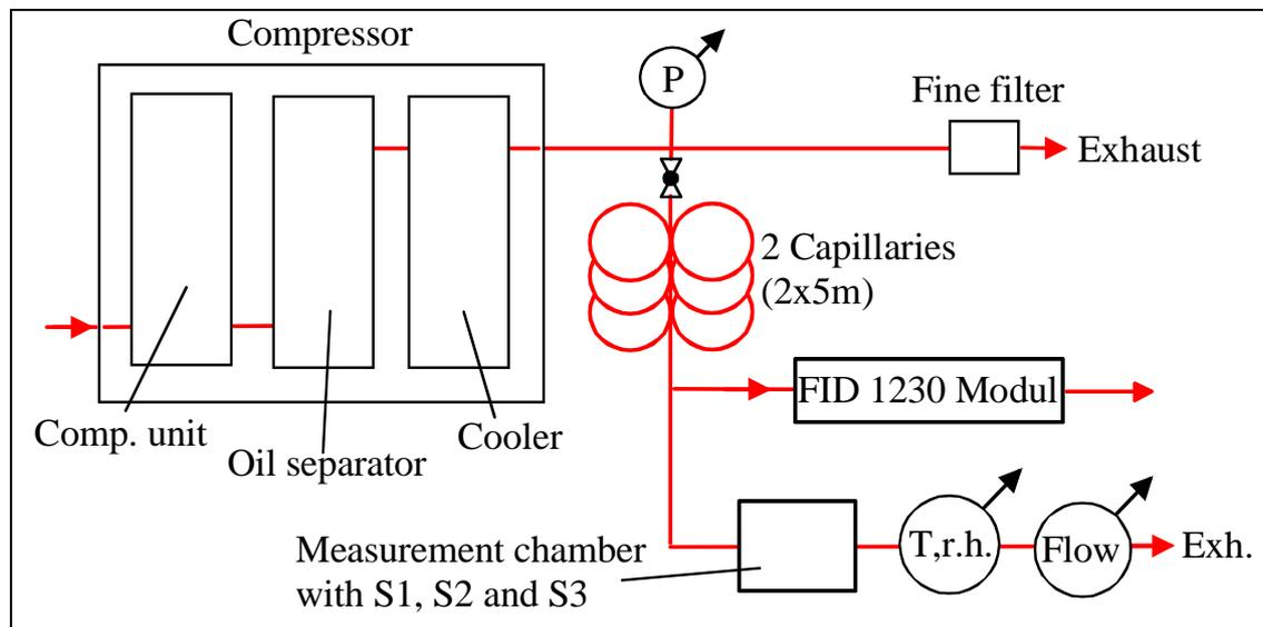
**Figure 21:** Schematic of the modified set up, as used at the end of the long term measurements, including the Testa FID „1230 Modul“ with an intake rate of ~ 18 ml/min.
