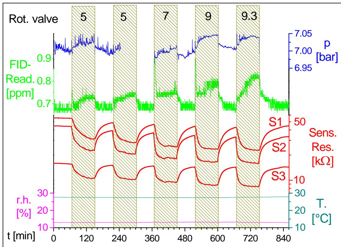
*Figure 37: Graphs of a measurement with increasing dosings up to the maximum exposure to oil aerosols with the set up (9.3 rotations of the needle valve). A discussion is given in the text.*
