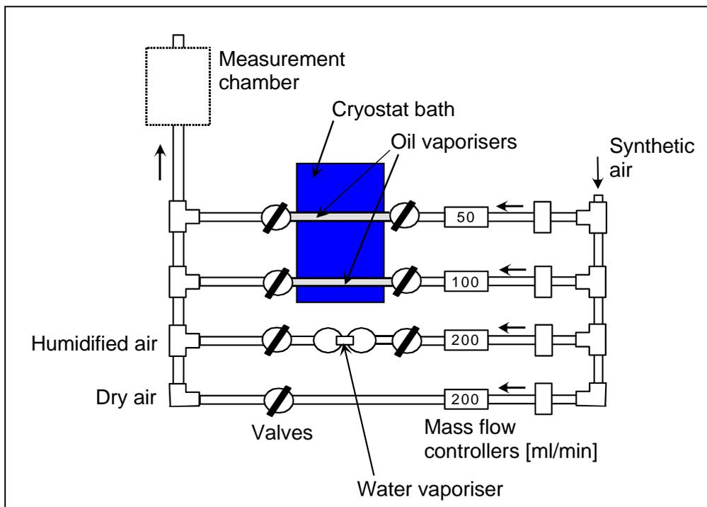
**Figure 11:** Gas mixing system as it was used for the measurements presented in 3.1.2.
