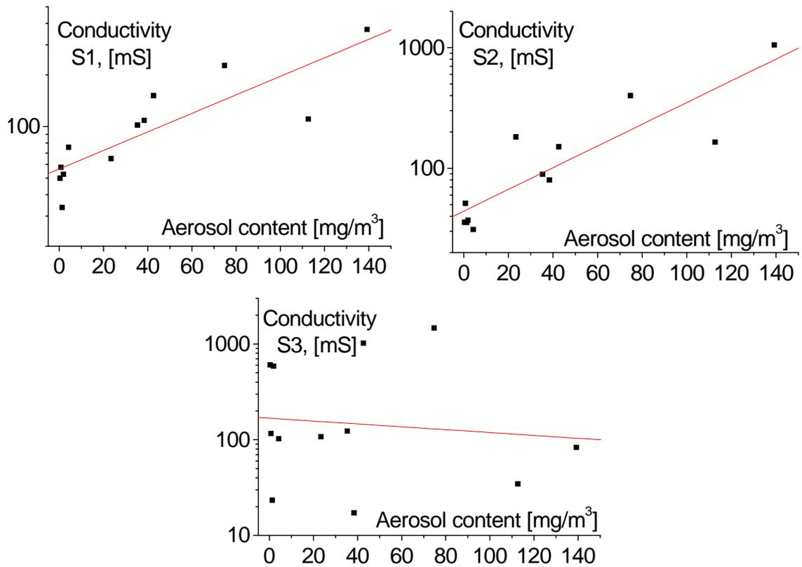
**Figure 42:** Correlation of gravimetrically investigated aerosol content and sensor conductivity (in mS). The respective trends are visualised by a linear fit.
