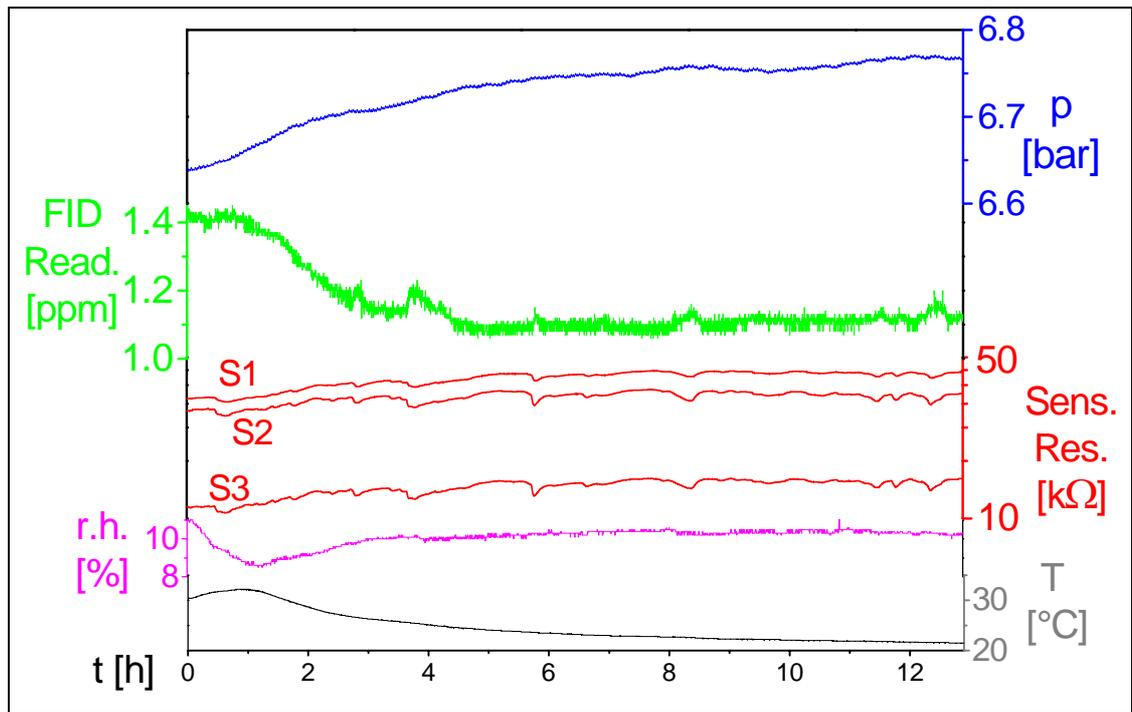
*Figure 25: Graphs of a measurement with changes of hydrocarbon content and correlated sensor response. Humidity stays constant within the time frame of the peaks of interest.*
