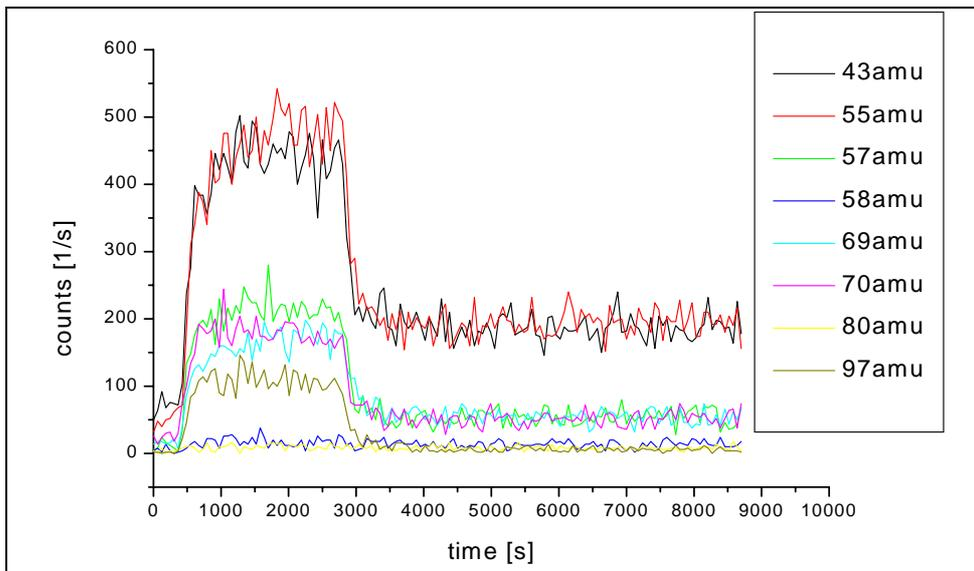
**Figure 13:** *Transient response of the RGA when exposed to 50 % air through an oil filled vaporiser at room temperature for 45 minutes. Balance and purging: synthetic air.*
