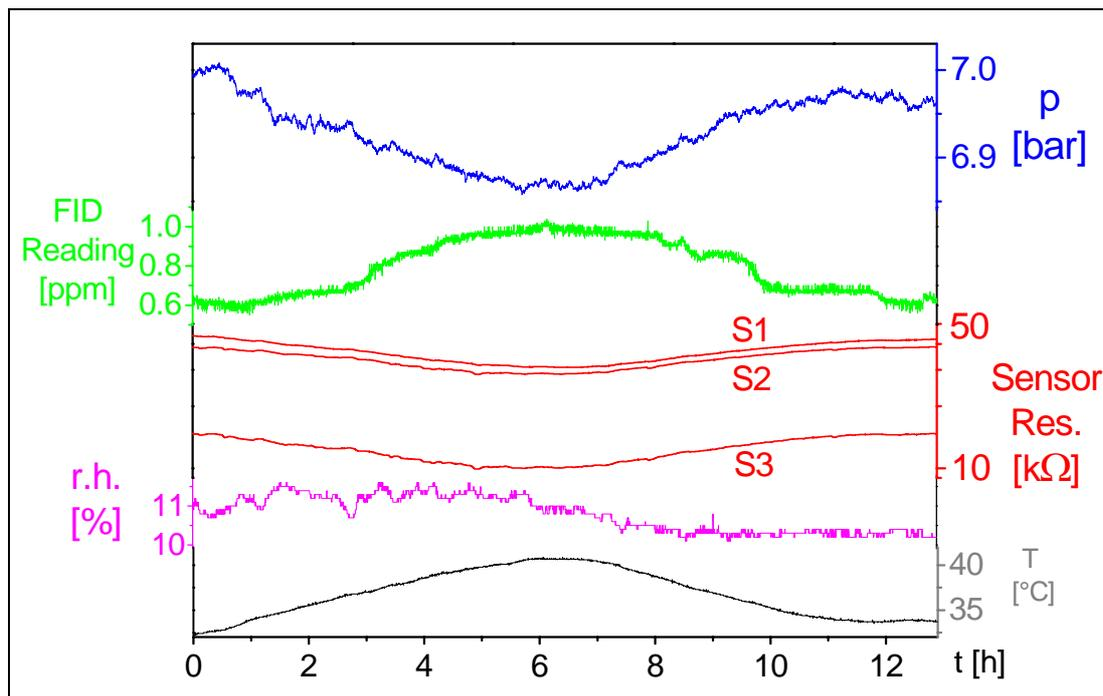
**Figure 23:** *Graphs of the measurements obtained on a warm day. The increase of temperature, given in the graph at the bottom is likely to be the reason for the change of the other parameters.*
