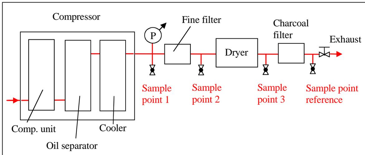
**Figure 15:** Schematic of the location of the sampling points within the filtering line for the measurements at different sampling points (3.2).
