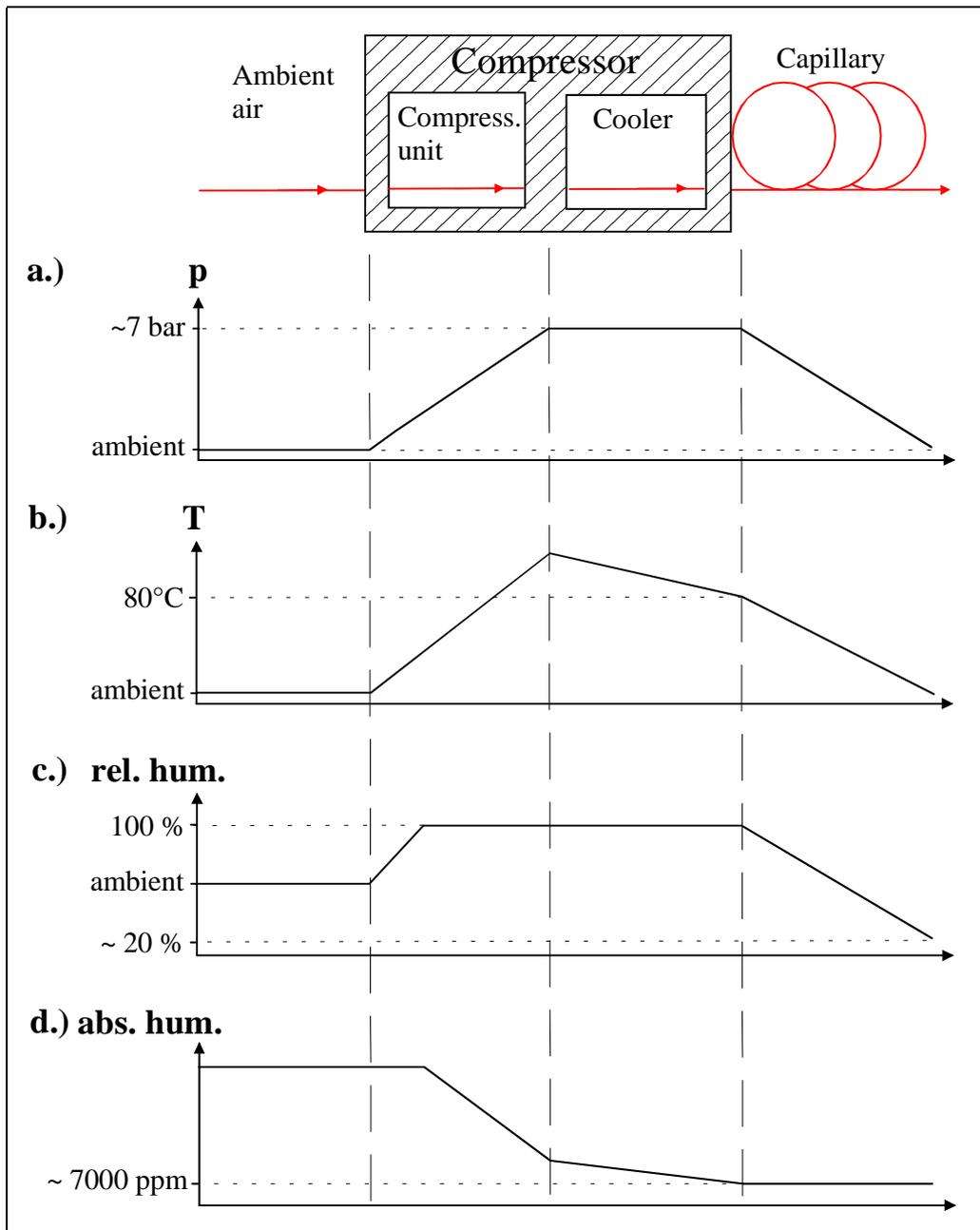
*Figure 31: Behaviour of pressure, temperature and humidity of humid ambient air when compressed by a compressor and expanded via capillary (Only the gaseous part is expanded). The numerical values are according to the set up and the conditions described in this chapter; the qualitative information can be applied generally. The absolute humidity here is a concentration per gaseous amount of substance, not per volume.*
