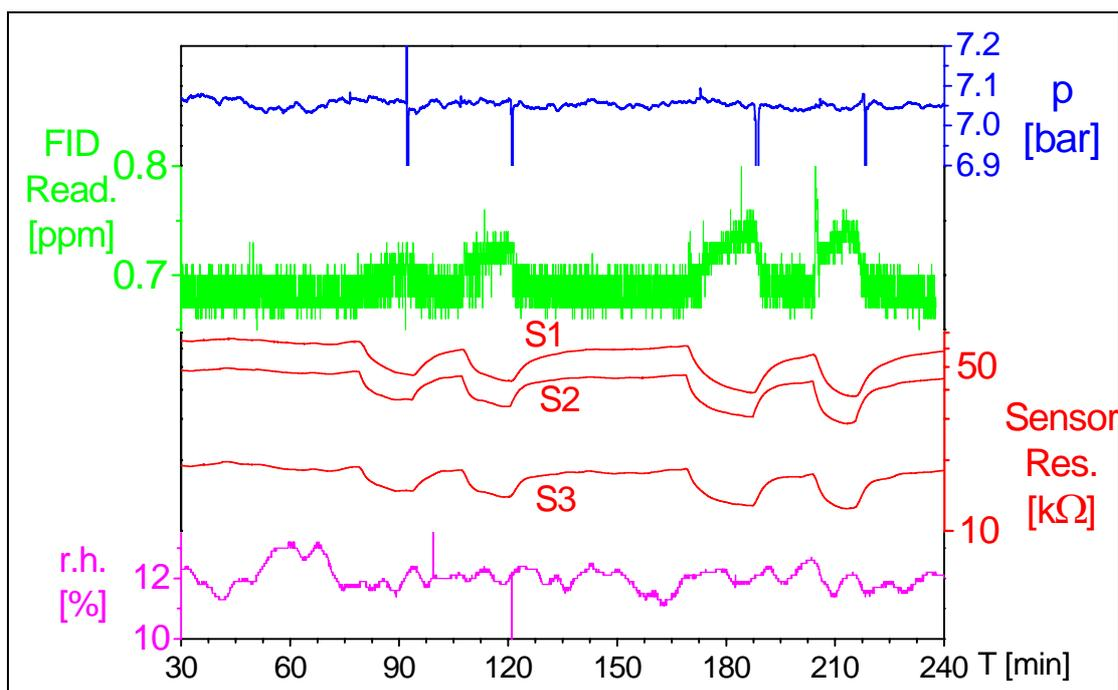
**Figure 36:** Graphs of a measurement with successive dosing of two, three, four and five rotations of the needle valve and intermediate baseline recovery.
