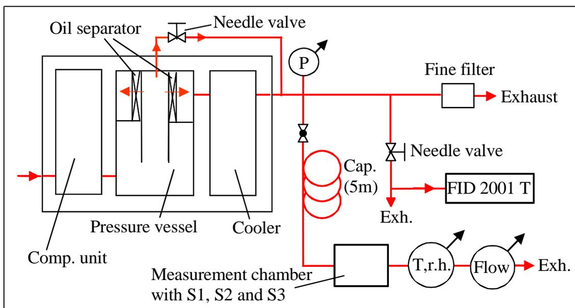
**Figure 32:** Schematic of the set up as used for the measurements with dosing of highly oil-contaminated air via bypass of the oil separator. The extent of dosing was controlled with a needle valve in the bypass. The tubing lengths are not proportional.
