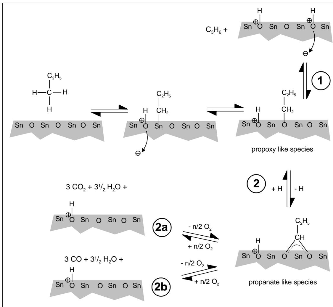
**Figure 8:** Mechanism of the reaction of propane on the heated  $\text{SnO}_2$  surface as far as known, focused on the oxidation of carbon. For the sake of simplification, all oxygen is shown as lattice oxygen, details are given in the text.
