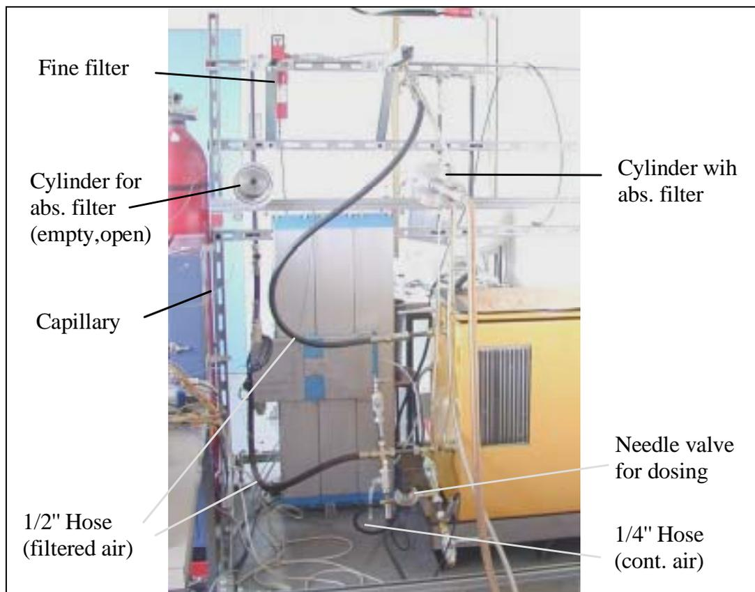
**Figure 34:** Photograph of the set up with a possibility for dosing of highly contaminated air and gravimetric referencing.
