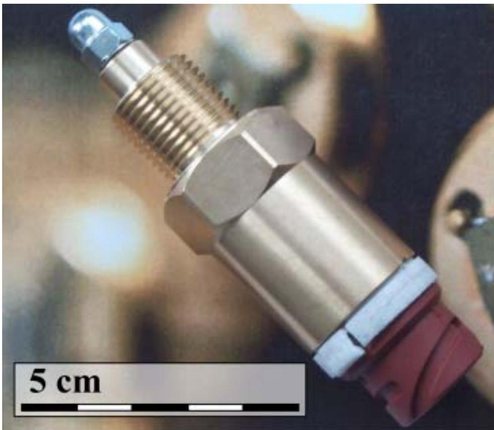
*Figure 44: Prototype of the residual oil indicator housing a five meter capillary, one MOX sensor and a PCB with readout, temperature regulation of the sensor heating and an A/D converter for complete digital control.*
