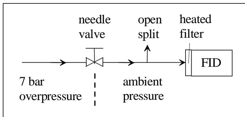
**Figure 9:** *Sample feeding as used for the Testa „2001 T“, in order to produce a flow of 750 ml/min sample gas.*
