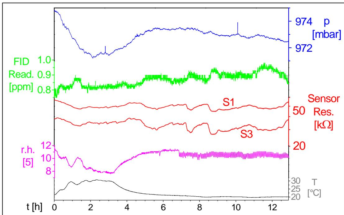
**Figure 24:** *Graphs of a measurement with monitoring of the ambient pressure. In the second half of the measurement, the humidity signal is corrupted because of coupling. Sensor S 2 was not measured. The sensor resistance is mainly correlated with the hydrocarbon content.*
