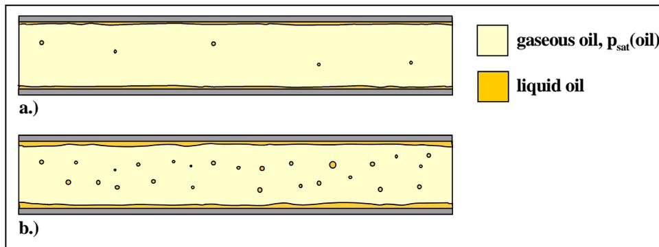
**Figure 2:** Schematic of the oil contamination of a tube downstream a compressor with a.) a properly working oil separator and b.) over aged oil separator with significantly reduced functionality.
