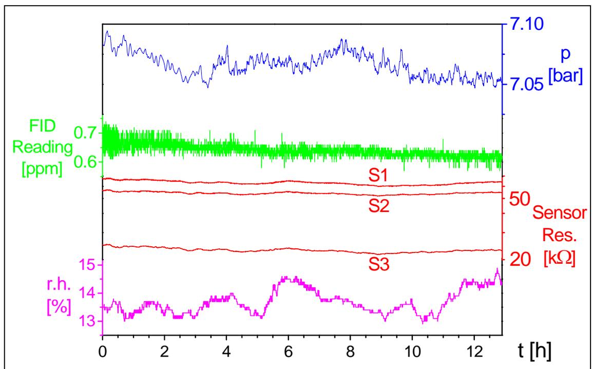
**Figure 22:** Typical graphs of a measurement on a cold day with stable values for all observed parameters. The change of humidity does not affect the sensor response. The temperature (not shown) stays constant.
