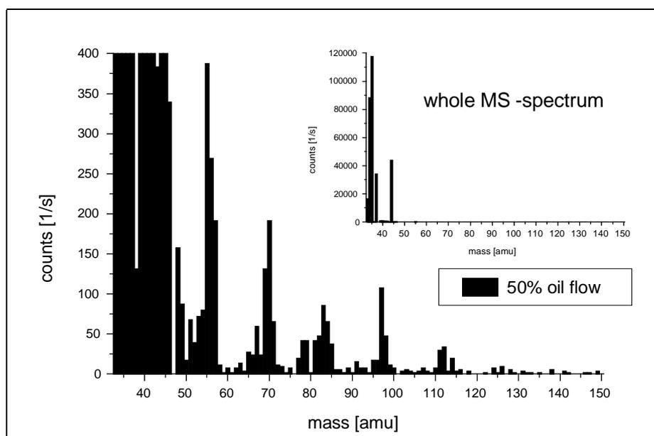
**Figure 12:** Difference mass spectrum of 50 % air through a vaporiser filled with used compressor oil at room temperature, residual: synthetic air.
