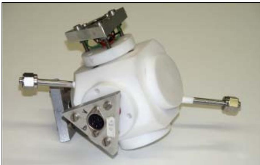
**Figure 7:** Cubic Teflon measurement chamber, equipped with three measurement holders.
