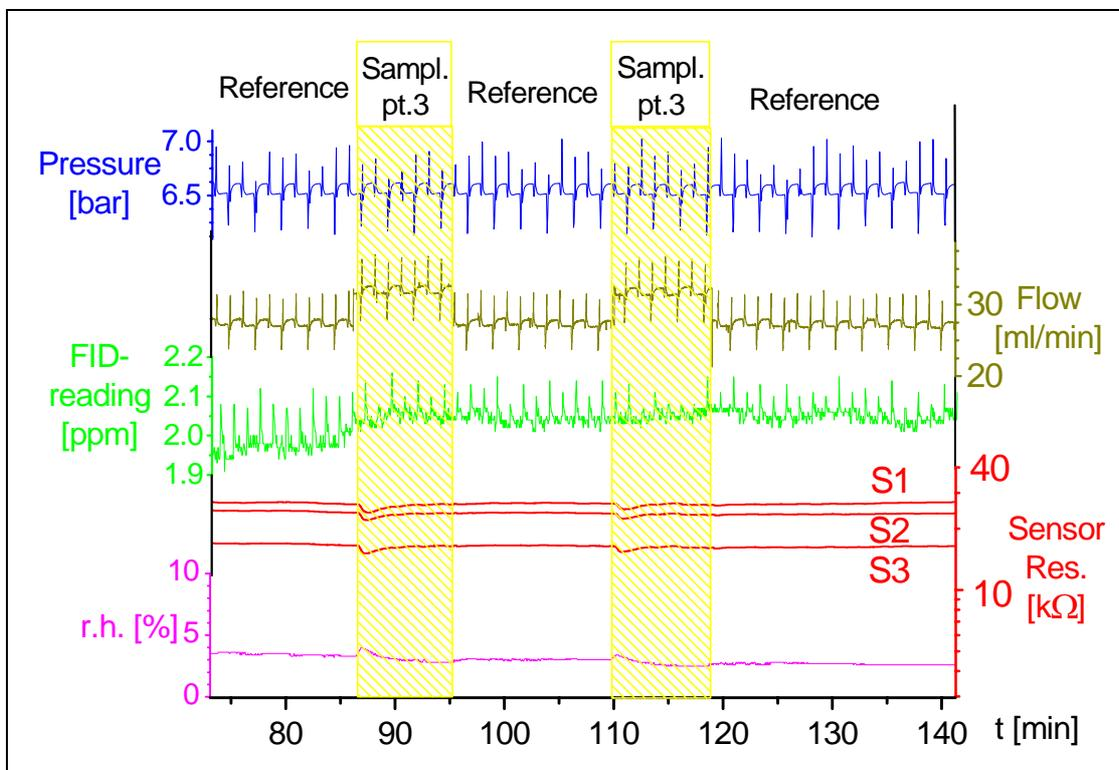
**Figure 17:** Graphs resulting from a measurement with switching between sample point reference and sample point three (see **Figure 15**), characterised by a charcoal filter in between. An interpretation is given in the text.
