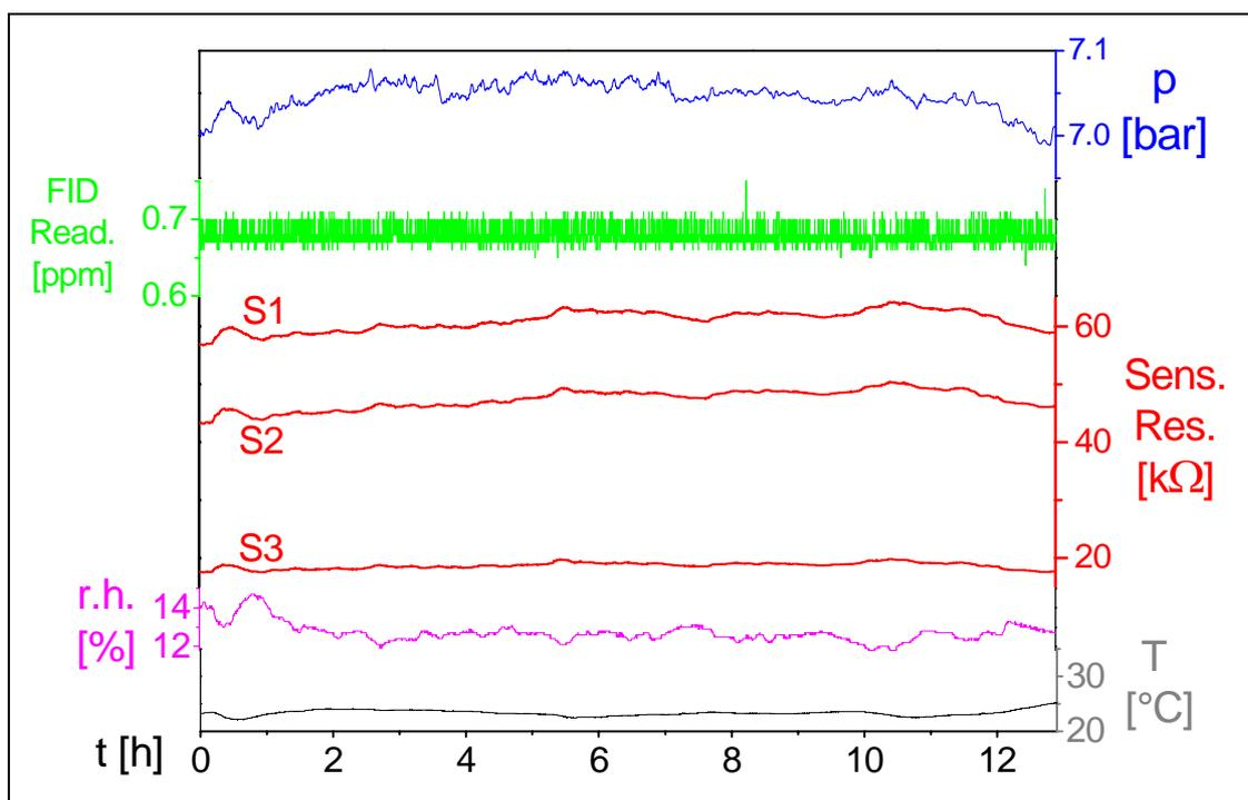
**Figure 26:** Graphs of a measurement with constant FID reading but correlated changes of pressure, humidity and sensor resistance. In contrary to most other figures the sensor resistance is displayed linear.
