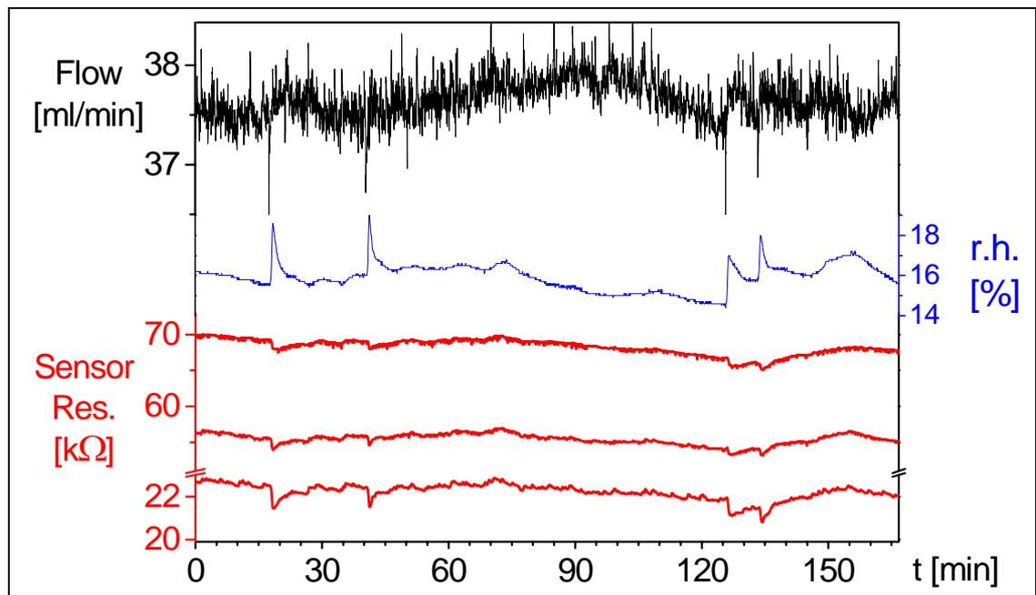
**Figure 29:** Typical graphs of flow, relative humidity and sensor resistance on a very humid day.
