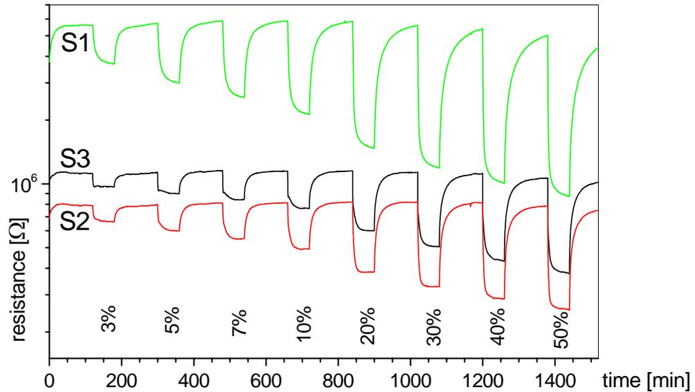
**Figure 14:** Sensor response towards exposure to increasing amounts of oil vapours in dry air, produced via vaporiser in a gas mixing system.
