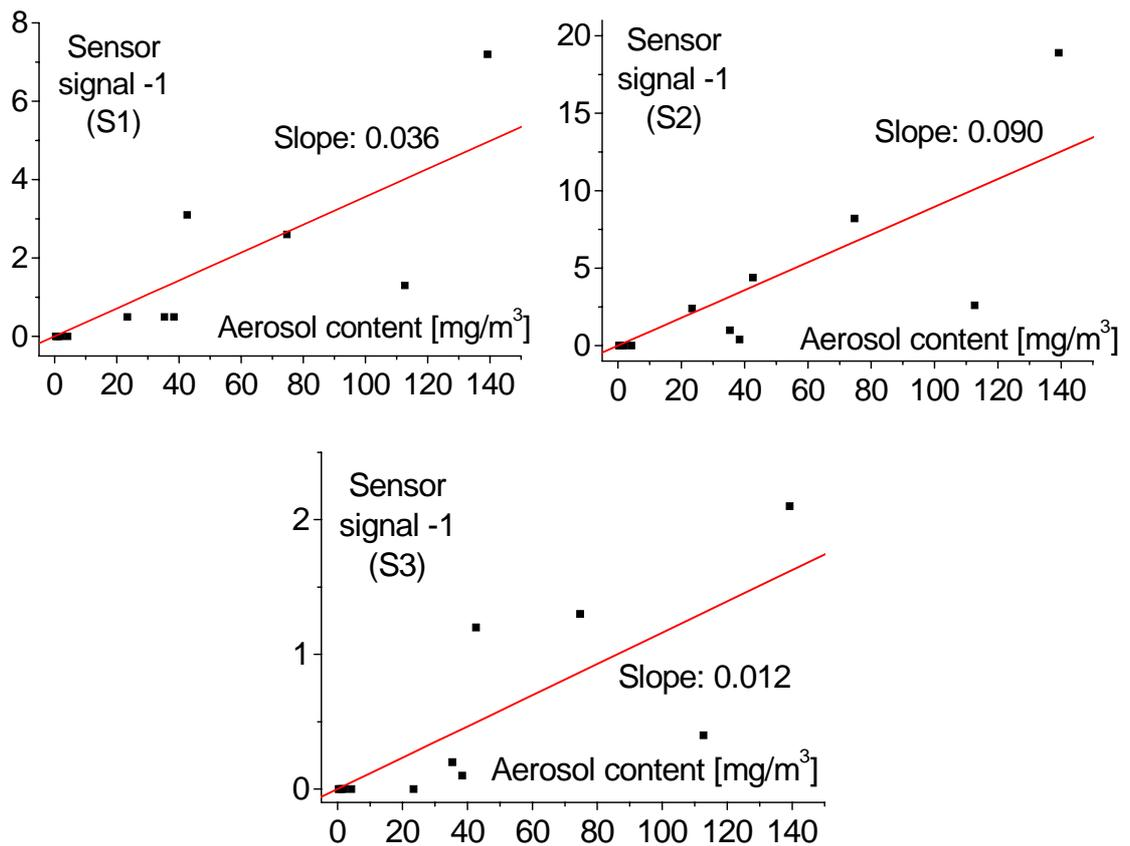
**Figure 41:** Correlation of gravimetrically investigated aerosol content and sensor signals minus one. A linear fit with zero crossing was applied.
