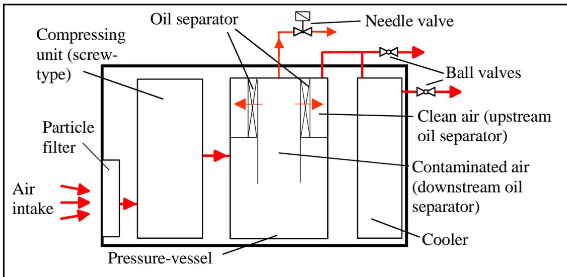
**Figure 3:** Schematic of the modified compressor: contaminated air can be sampled from an additional drain upstream the oil separator; a second additional drain was mounted between the pressure-vessel and the cooler. The oil separator is shown cross-section-like in order to illustrate the flow from inside to the outside.
