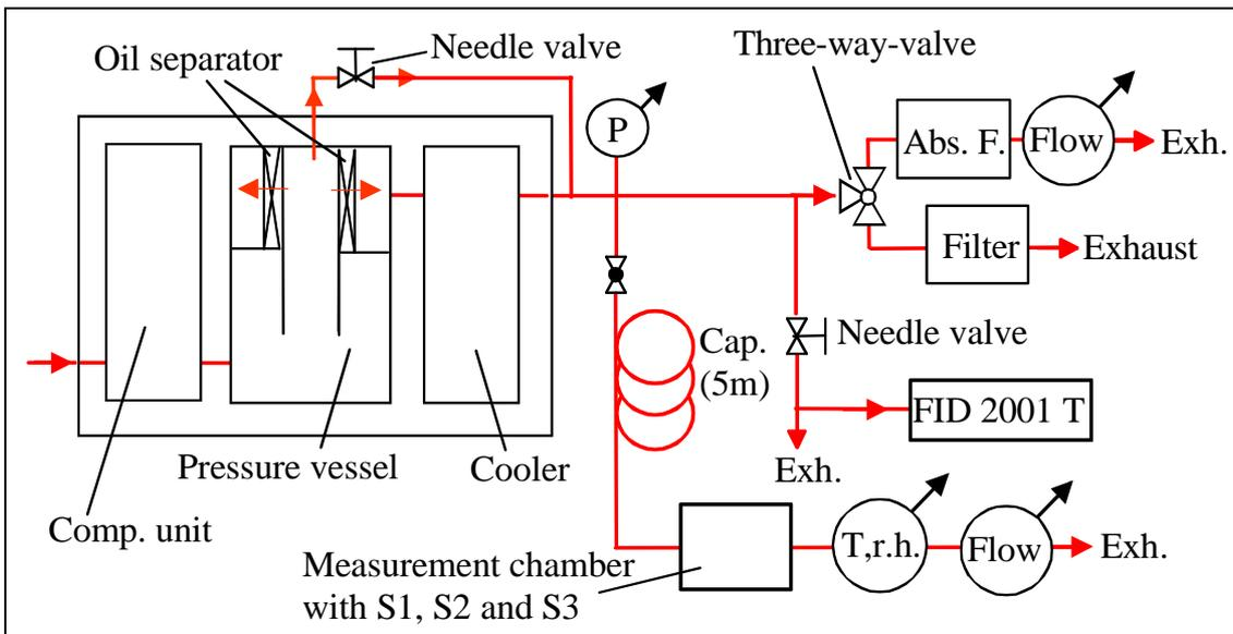
**Figure 33:** Schematic set up with possibilities for the dosing of highly contaminated air and gravimetric referencing with absolute filters (Abs. F.).
