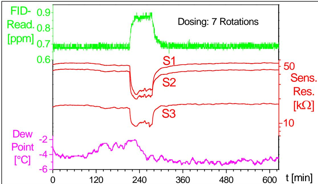
**Figure 38:** Graphs of a measurement with strong humidity interference. The sensor response to the dosing is superposed by a humidity response.
