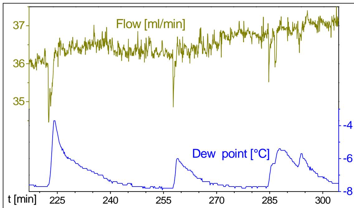
**Figure 30:** Magnified graphs of flow (smoothed by moving average of three values) and absolute humidity on a very humid day. A discussion is given in the text.
