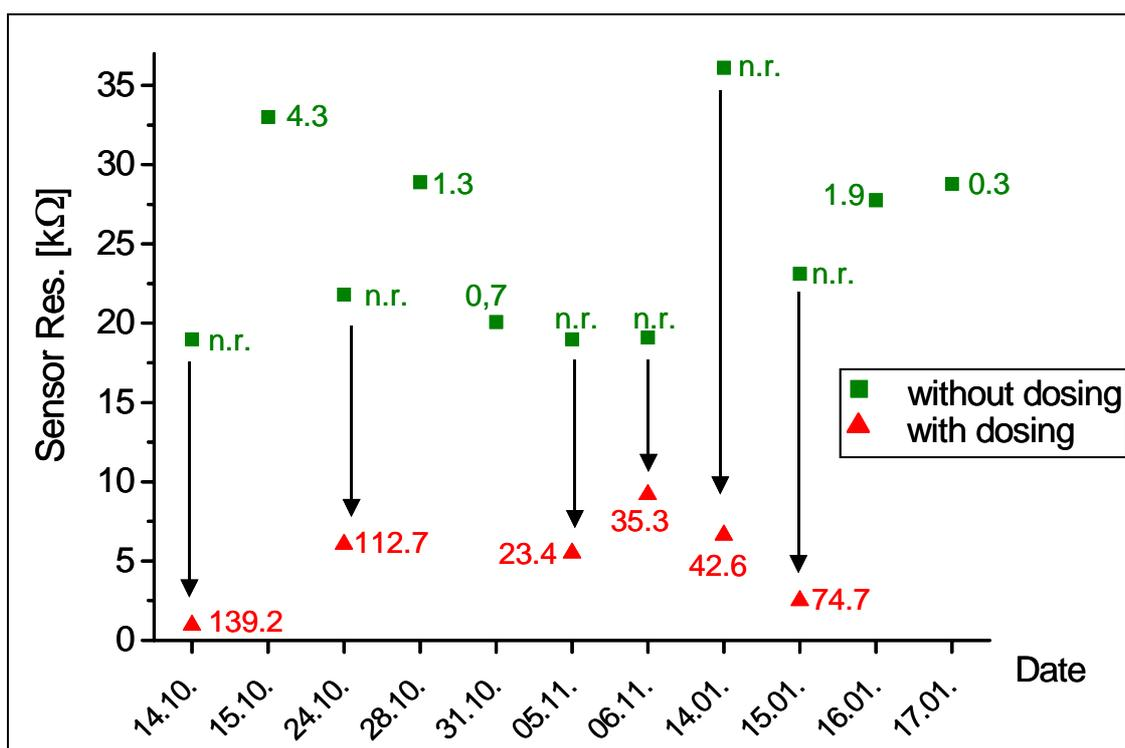
**Figure 43:** Visualisation of the absolute sensor response of S 2 due to dosing and gravimetrically referenced baseline resistances. The baseline before dosing was not gravimetrically referenced (*n. r.* in the graph).
