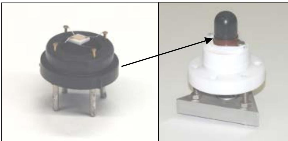
**Figure 6:** Pictures of one sensors and its socket (black, left side) and a Teflon measurement holders (left side), equipped with sensor and socket (black, with black cap on sensor socket).
