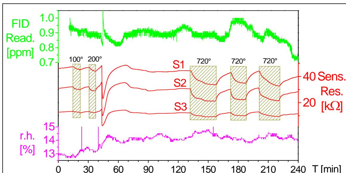
**Figure 35:** *Graphs of the first measurement with dosing of highly contaminated air via bypass. The peak between ~40 and 50 minutes resulted from a short shut off (< two minutes) of the compressor. In this diagram, the opening of the needle valve is indicated in degrees.*
