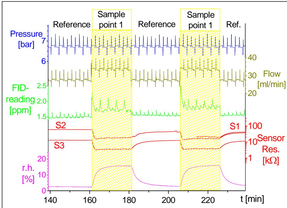
**Figure 19:** Graphs resulting from a measurement with switching between sample point reference and sample point one (see **Figure 15**), characterised by a fine filter, a dryer and a charcoal filter in between. An interpretation is given in the text.
