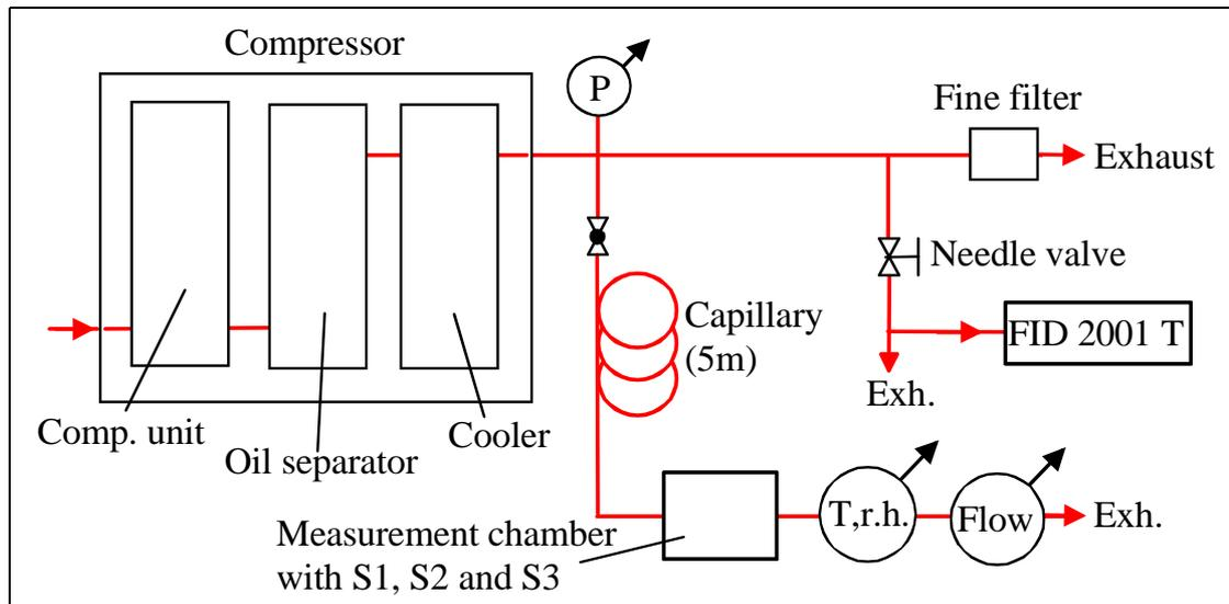
**Figure 20:** Schematic of the second compressor set up, as used for the long term measurements.
