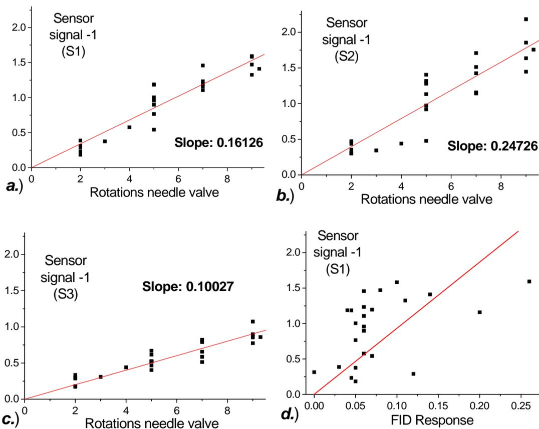
**Figure 39:** Correlation between the sensor signals and **a.) – c.):** rotations of the needle valve, **d.):** FID response.
