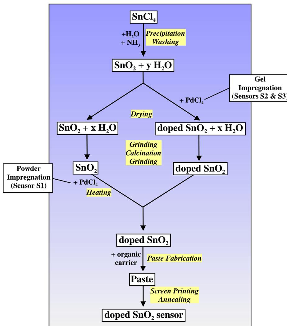
**Figure 4:** Flow chart of the preparation of the three SnO<sub>2</sub> thick film sensors used in this work. The difference in performance is due to the different methods of doping, (gel impregnation or powder impregnation) and the extent of doping.
