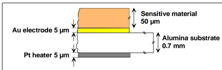
**Figure 5:** Cross section of the sensor, used for the measurements. The three sensors differ in characteristics of the sensitive material, caused by different dopings.
