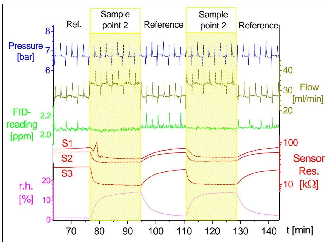
**Figure 18:** *Graphs resulting from a measurement with switching between sample point reference and sample point two (see **Figure 15**), characterised by a dryer and a charcoal filter in between. An interpretation is given in the text.*
