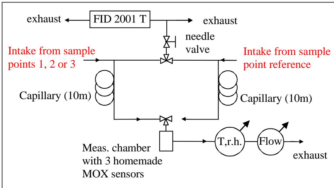
**Figure 16:** Assembly of the measurement devices and sample feedings of the measurements at different sampling points (3.2). Both capillaries have been continuously flown through.
