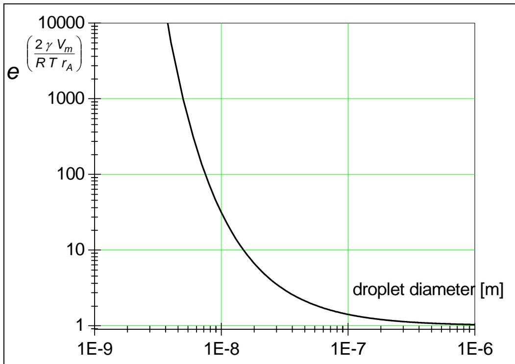
**Figure 10:** Graph of the exponential factor  $e^{\left(\frac{2\gamma V_m}{RT r_A}\right)}$  in dependency of the aerosol diameter  $d = 2 r_A$ .
