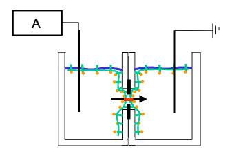
**Fig. 2:** Bilayer set up used for channel recordings. The lipids are put onto an aqueous subphase (blue) in both sides of the chamber and raised to cover a small aperture in a Teflon film (thick black bars between the two chambers). Inserted ion channels (red) allow the ion flux (arrow) which can be registered with the electrodes. The left electrode is connected to the amplifier (A). This side is called the cis side in this study. The other chamber is grounded and called trans side.
