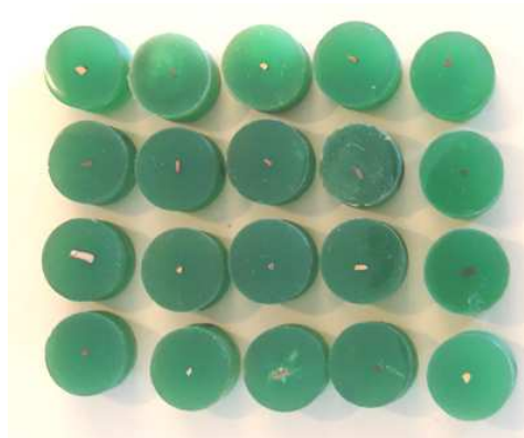
Abb.5.47. 20 Proben in Epoxidharz
