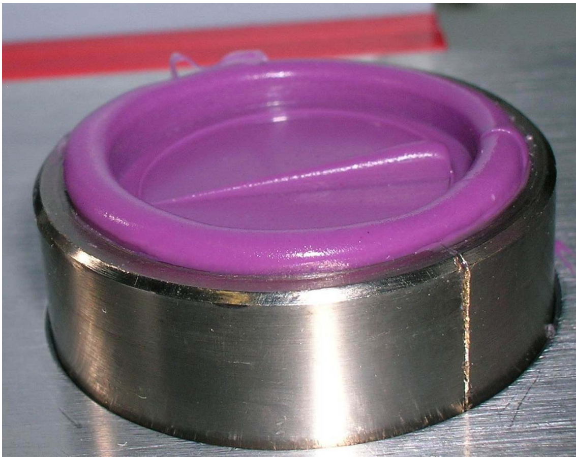
Fig 20: Sharkfin of Aquasil ULV® (type 2) at 81s.
