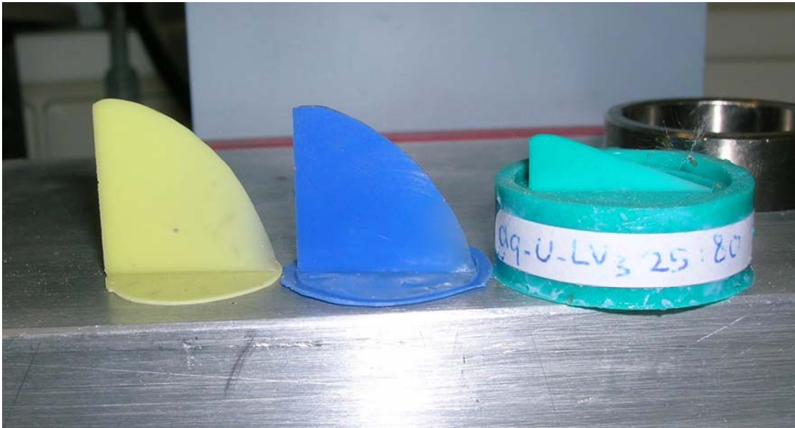
Fig 19: Sharkfins of Aquadyn light® on the left, Permadyne Garand 2:1® in the middle and Aquasil ULV® on the right at 26s.
