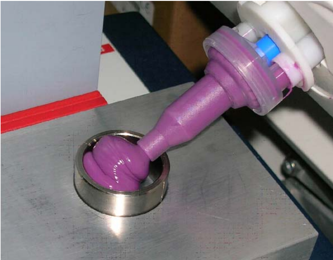
Fig 10: Filling of the receptacle with material, the stopwatch was started.
