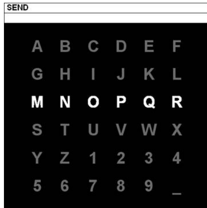
Figure 4.1: The character matrix display in the P300 speller paradigm. In this example, the users task is to spell the word "SEND".
