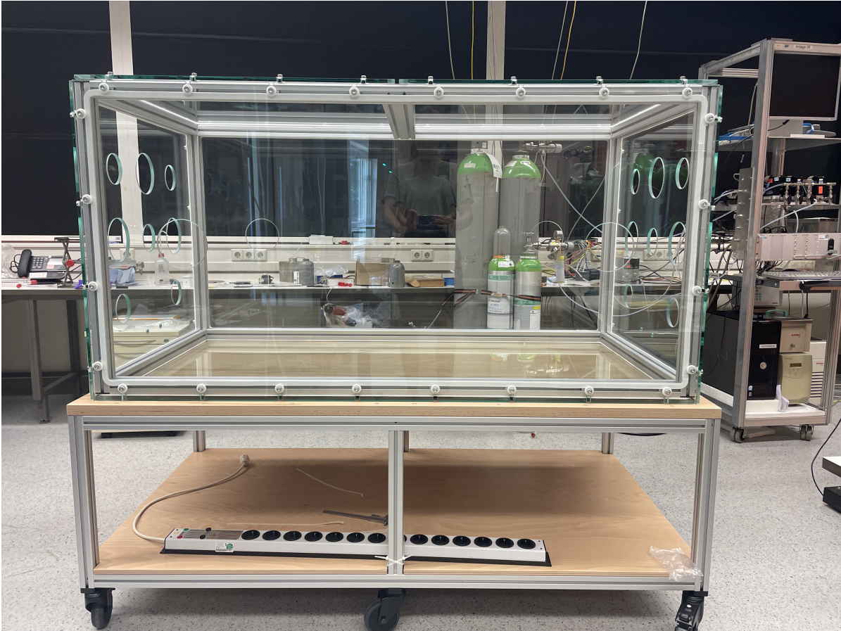
Figure 3.3: Photograph of the test volume enclosed by plates of glass on the mobile bench. The PTFE sealing was later exchanged with a broader sealing, covering the full width of the aluminum profile.
