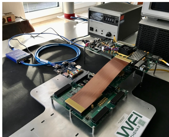
Figure 84: Real-time performance testing setup operating at IAAT. The FP-MB receives data from the Virtex 7 development board (top) through a flex-rigid PCB connector. Output data is received through the SpW interface for its analysis.
