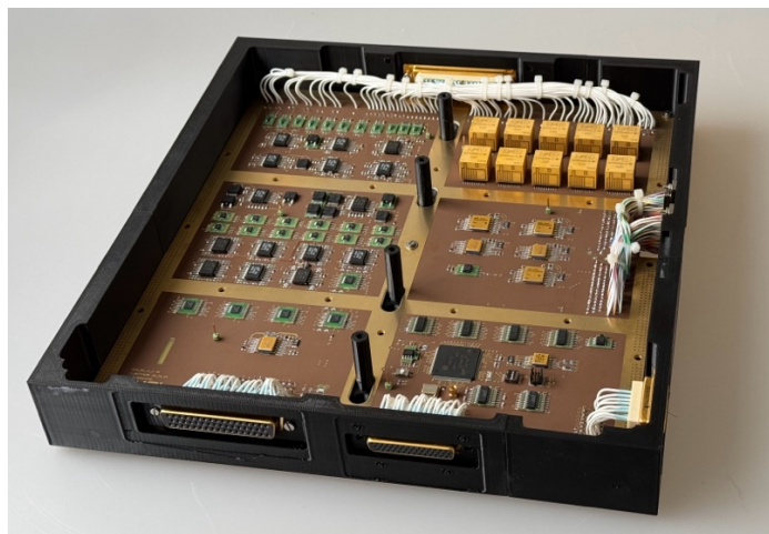
Figure 14: Engineering Model of the Power Conditioning Module. To reduce development costs, a mix of space qualified and commercial equivalent components are used.
