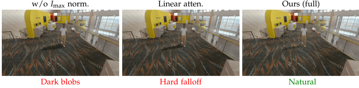
Figure 9.5: Visual ablations. Without I_{\max} normalization (left), large anisotropic Gaussians cast disproportionately dark shadows. The linear attenuation model (middle) produces harder shadow falloff than our full exponentiated model (right).
