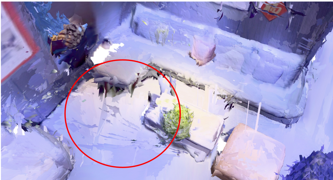
Figure 8.9: VGGT mesh reconstruction from monocular video. The underlying mesh contains blocked paths and significant noisy structures.
