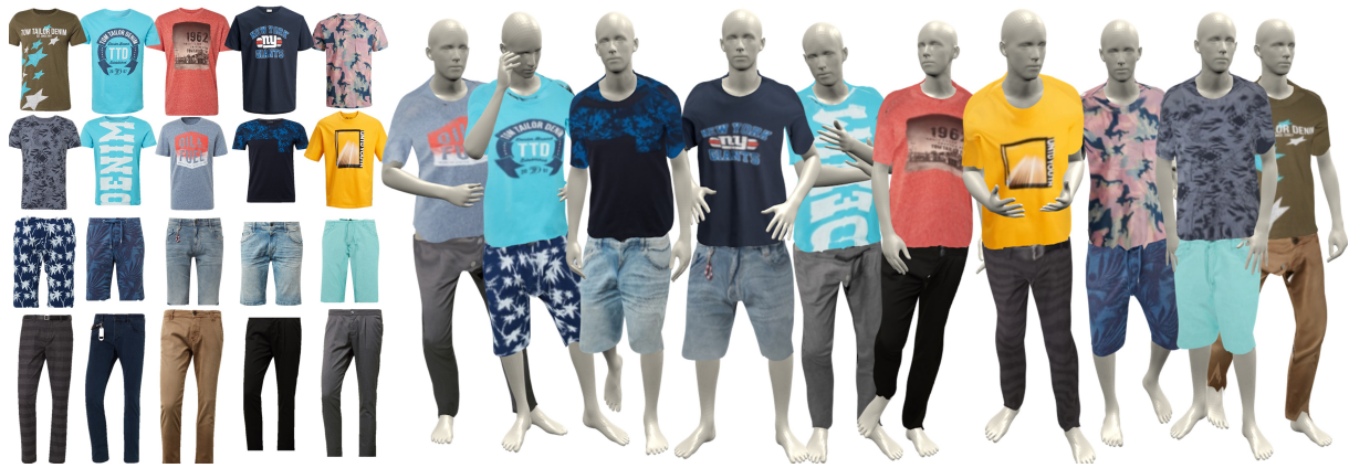
Figure 4.1: Real-time texture transfer to 3D garments. Our model Pix2Surf digitally maps the texture of online retail store clothing images to the 3D surface of virtual garment items, enabling 3D virtual try-on in real time.
