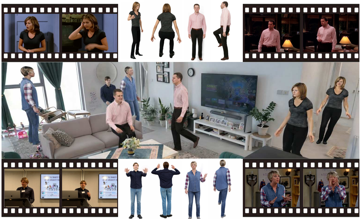
Figure 10.1: AHOY reconstructs animatable 3D avatars from occluded YouTube video. Given a monocular YouTube video with occlusion, AHOY reconstructs a complete, animatable 3D human avatar using video diffusion priors and 3D Gaussian Splatting, enabling photorealistic human animation within 3D scenes.
