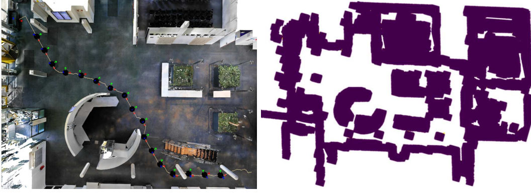
Figure 6.4: Scene map and path planning. Right: scene point cloud projected down to get a map of the scene. Left: A* trajectory with keypoints in black and tangents in red.
