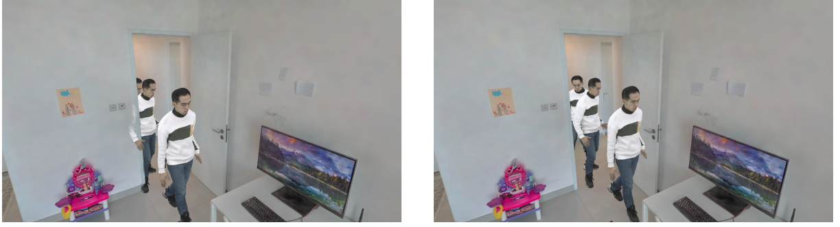
Figure 8.4: Effect of the egocentric walkability grid (Sec. 8.3.2). Left: without the walkability map, the RL policy lacks local obstacle awareness and generates motion that passes through the desk. Right: with the walkability grid extracted from scene Gaussians, the avatar correctly avoids the obstacle.
