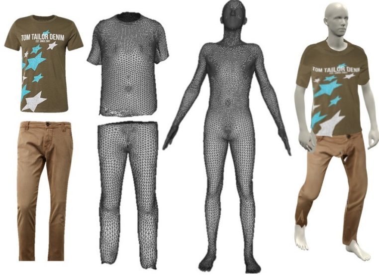
Figure 4.2: Automatic texture generation for 3D garments. Given online retail store images, our method produces textures for pre-defined garment templates that can be used to virtually dress SMPL [Loper et al., 2015] in 3D.
