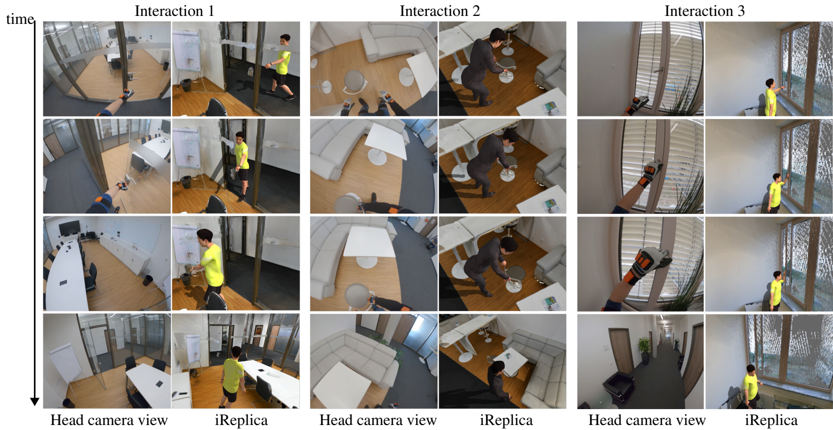
Figure 5.10: Qualitative results. We show three examples of human interaction, pairing the head-mounted camera view with the interaction modeling achieved by iReplica. The object is not always visible during the interaction (Interaction 1), hand grasping can be difficult to understand from the camera (Interaction 2), or object occludes a majority of the first person view (Interaction 3). By relying on human-centric contact detection, iReplica achieves reliable modeling in all these challenging scenarios. Please see our video for more results.
