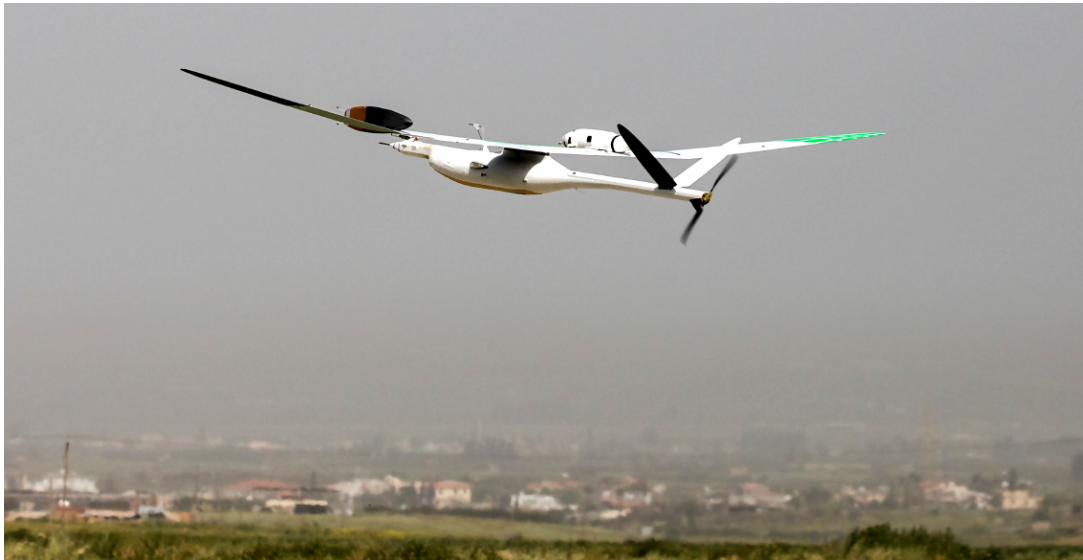
Figure 2.6: The MASC-3 in flight, with its scientific payload mounted in the front and both Pods on the wings. Photo by Christos Keleshis.
