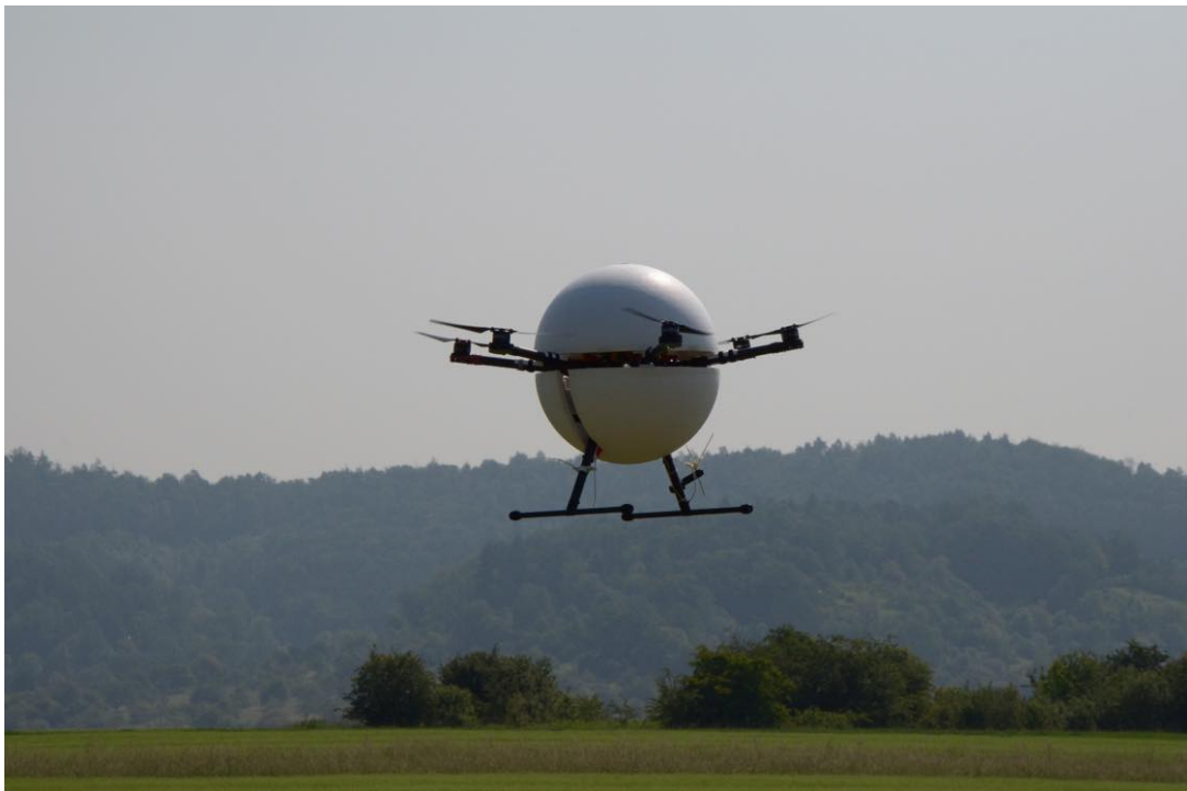
Figure 2.5: The MASC-MC, which is an altered version of the DJI S900 commercial frame, in operation. The autopilot system, batteries and sensor electronics are located inside the two styrofoam domes, while an opening at the upper dome's top allows for aerosol particle sampling. Photo by Martin Schön.
