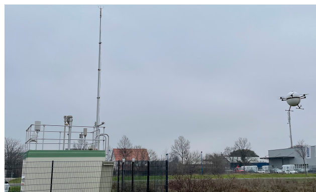
FIG. 4. The S900 in flight (right) next to Mannheim-Nord station (left). The sensors, including the aerosol particle measurements from the Fidas 200, are located at the roof of the station. The distance between the S900 and the station was maintained between 7 and 12 m for safety reasons, and for the UAS downwash to leave the station's measurements unaffected.
