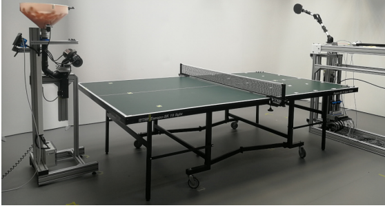
(a) Setup with the ball launcher (left) and the robot arm (right).
