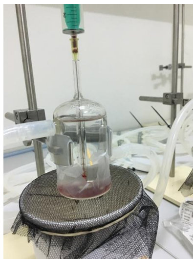
Fig. 10 : Direct membrane feeding assay using P. falciparum field isolate. The system is connected to a 37°C water circulation to avoid gametocytes ex-flagellation and allow the parasite transmission to the mosquitoes in a cup. The blood was gently put into the
