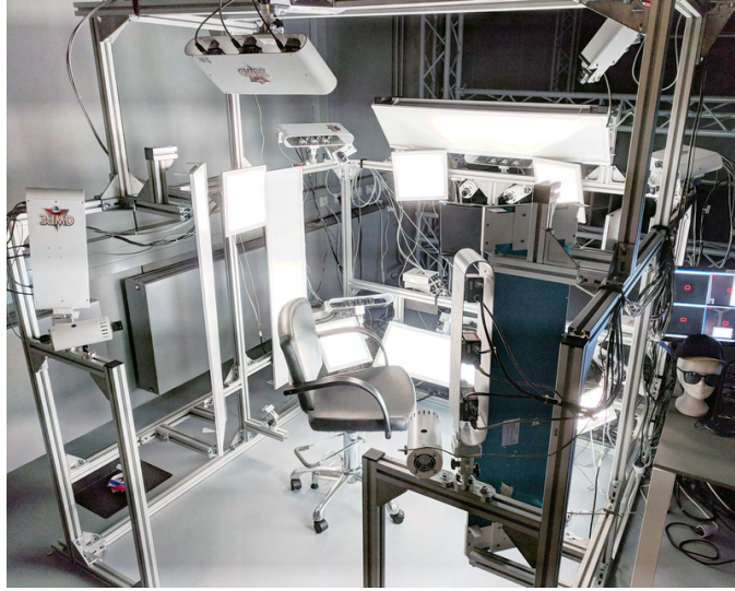
Figure 4.5: Head Scanner: An overview of the head scanner. In contrast to the the full body scanner, the head scanner has a limited scanning volume which is focused on the subject head/neck region. The setup is sufficient for high-resolution capture of the human head including subtle deformation due to facial expression. However, the scanning setup is limited to capture the full range of motion of the head relative to the body.
