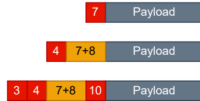
Fig. 13. Headers after discovering nodes 7, 8, and 10 in the example. SEET headers are depicted red while local bitstrings are depicted orange. Numbers indicate the destinations of the respective header.
