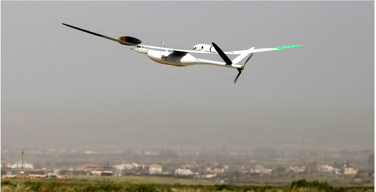
FIG. 1. MAS-C3 directly after takeoff, flying away from the camera, at the Unmanned System Research Laboratory (USRL; Kezoudi et al. 2021b) airfield of the Cyprus Institute, near Orounda, Cyprus. The atmospheric charge measurement pod is mounted on the left wing, while the OPC-Pod is mounted on the right wing. The meteorological sensor payload is on the nose of the aircraft. The low visibility in the background is due to a Saharan dust event. Photo by Christos Keleshis, Cyprus Institute.
