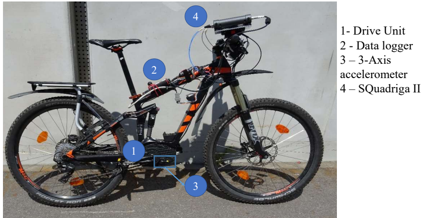
Figure 5.16: Setup used for the data generation and collection.
