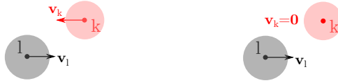
Figure 11.2: Two motion scenarios, both having the same category, i.e., S_{14}(\text{DC}_-) , in the motion representation Motion-RCC. The fact that in the second scenario the entity k is motionless is no hindrance for a scenario categorization.
