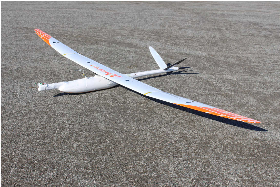
Fig. 2 The Multi-Purpose Airborne Sensor Carrier, version 3 is a UAS for meteorological measurements in the atmospheric boundary layer. The image shows the UAS with its sensor compartment (Rautenberg et al. 2019). Picture taken by Barbara Altstädter
