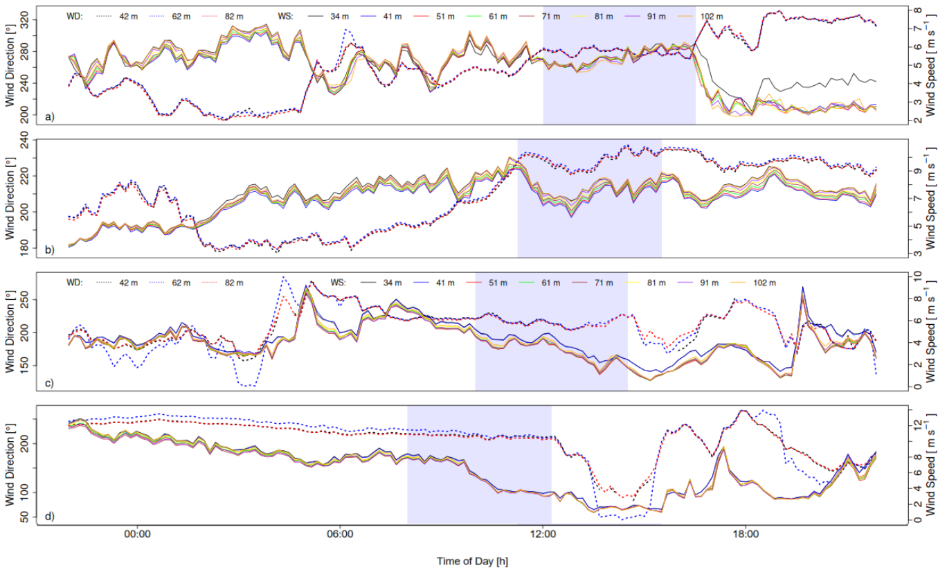
Figure 6 FINO1 data for wind speed and wind direction for the four measurement days in July 2020 and 2021 at various tower levels. The wind speed (solid lines) and wind direction (dotted lines) for the measurement days 14.07.2020, 23.07.2020, 27.07.2021 and 30.07.2021 are shown in sub figure a) to d), respectively.
