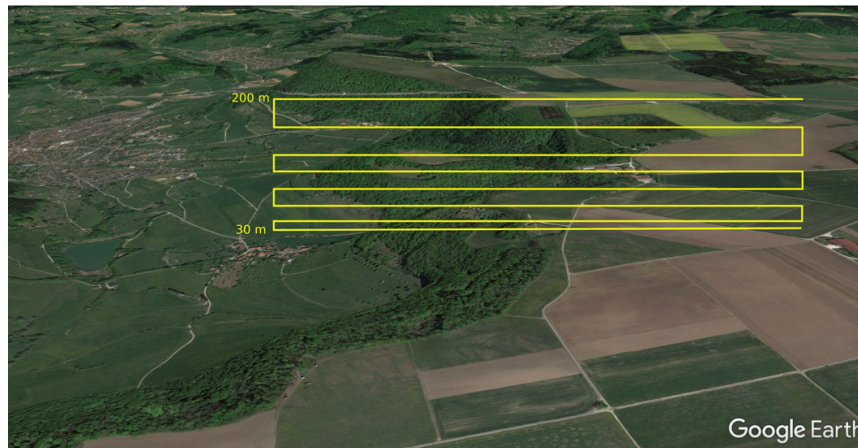
Fig. 5 Flight paths between 30 and 200 m above the plateau. The escarpment is facing west. Source of the satellite image: Google
