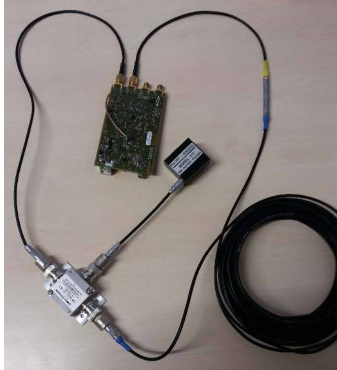
Figure 2.18: Shows a picture of a test setup for the SP-test. One can see that the pulse from the pulser is split via a power splitter. Additionally one split signal is delayed by around 50 ns before both are digitized in the V3.
