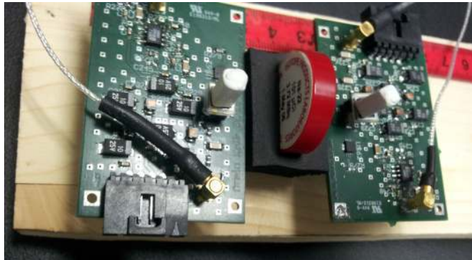
Figure 2.20: Shows a picture of the CRT-test with APDs coupled to a scintillator-crystal (second category).
