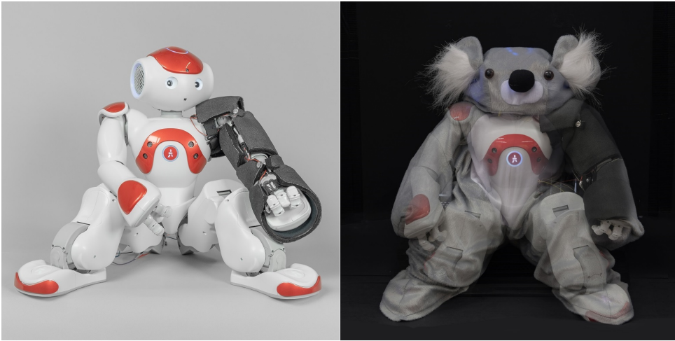
Figure 4.1: Left: Custom tactile sensors were built from fabric and foam to wrap around the four rigid segments of NAO’s arm. Right: As seen in this photo-merge, the sensors are secured on top of the robot’s plastic exterior and are hidden underneath a soft koala suit to create the robot companion HERA. Photos redistributed from [24] under a Creative Commons License, CC BY.
