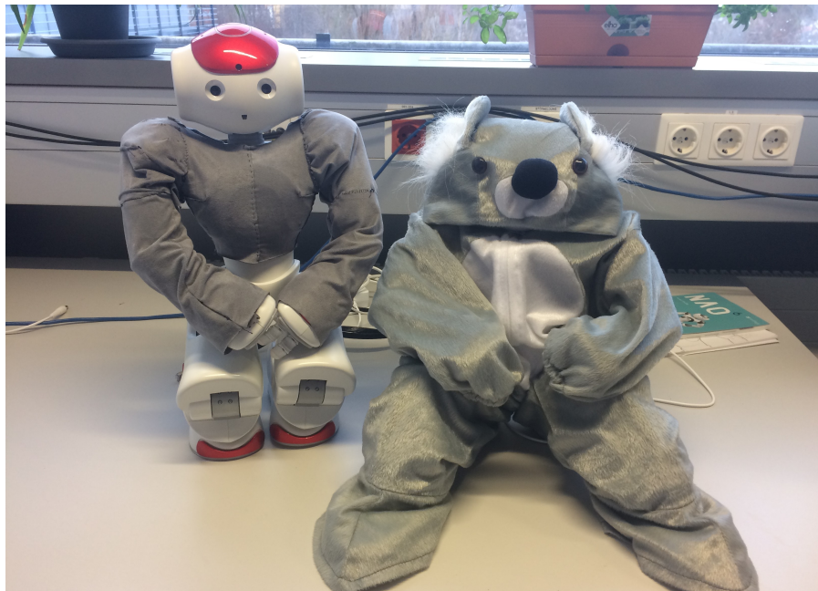
Figure 3.1: The prototype robot companion for children with autism that was presented to the therapists in our interview study. It is a NAO robot (SoftBank Robotics); the NAO robot shown on the left is wearing a thin fabric shirt, and the one on the right is enclosed in a soft koala suit. Photo redistributed from [22] under a Creative Commons license – Attribution 4.0 International (CC BY 4.0).
