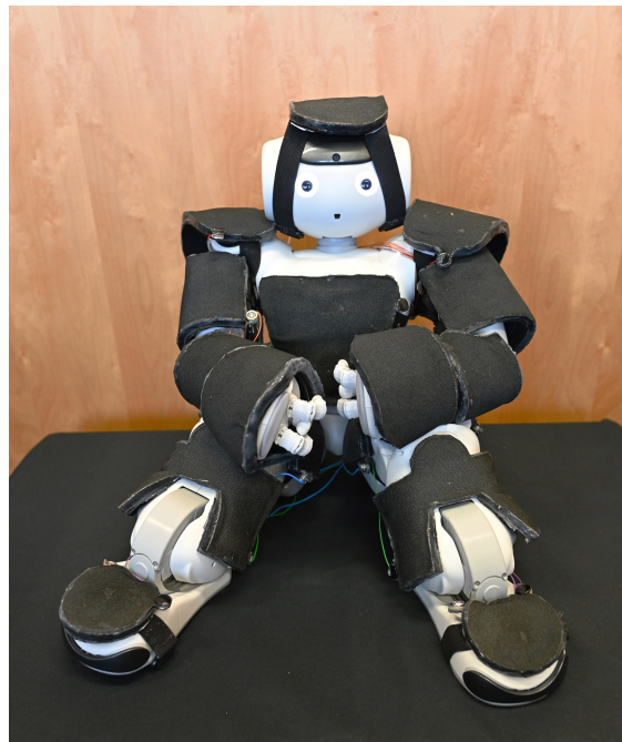
Figure 6.5: A view of all the sensors hidden under HERA’s koala suit. The inner NAO robot is covered with sixteen improved sensors, which provide HERA with whole-body tactile sensing. Moving joints were not covered to avoid pinching.
