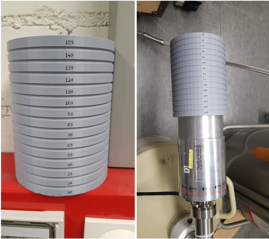
Figure 7.2: Left: Centering ring for the HPGe detector. It perfectly fits the outside of the HPGe detector and the inside of the PET scanner. It is made from PLA in a 3D printer and has markings on the outside indicating how far the HPGe detector was inserted into the PET scanner. Right: Centering ring mounted onto HPGe detector.
