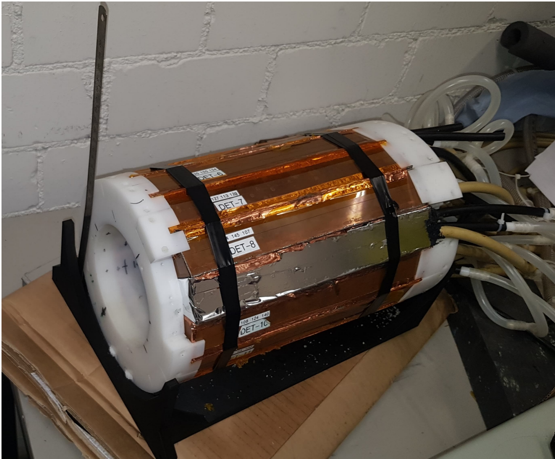
Figure 6.2: Picture of the PET scanner. The metal ruler inserted for scale has a length of 30 cm.
