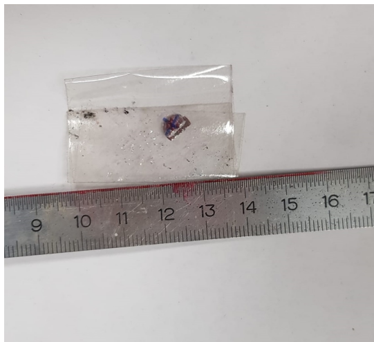
Figure 6.4: Picture of the point-like ^{22}\text{Na} source. It has an activity of about 33 kBq and was manufactured by Eckert und Ziegler.
