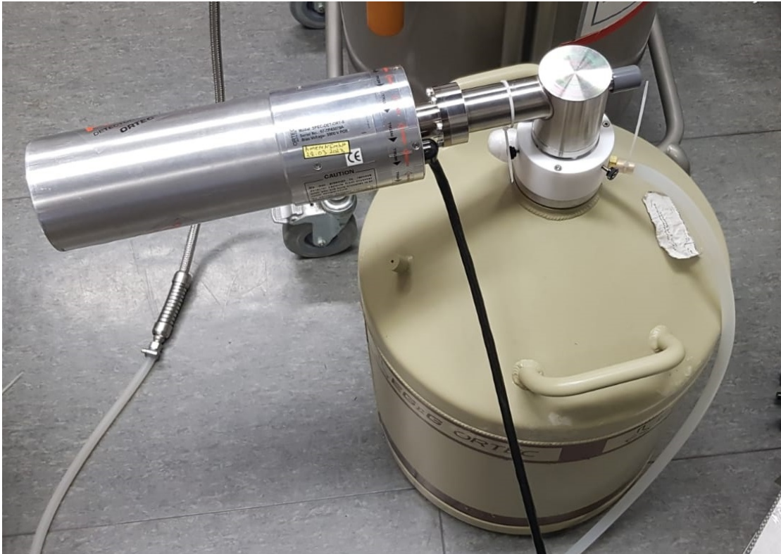
Figure 6.17: Picture of the used HPGe detector. It is mounted in an ORTEC PopTop cryostat and attached to a 301 Dewar.
