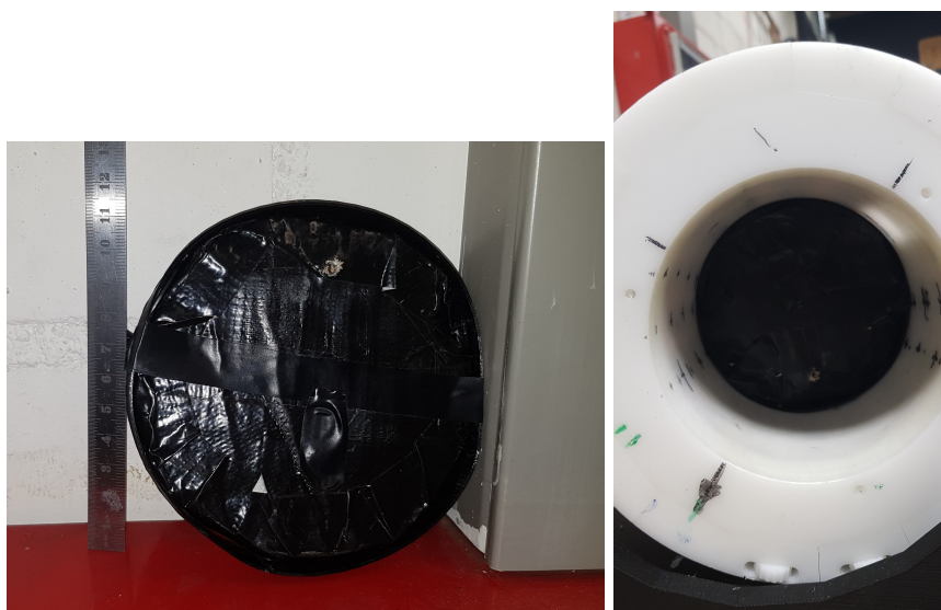
Figure 7.3: Left: Circular collimator used for the measurement. It is made of lead with a thickness of 15 mm and has a hole with a diameter of 5 mm about 30 mm from the outer edge. Right: Collimator placed in the PET scanner.
