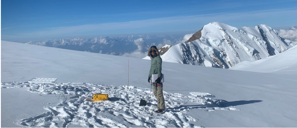
Figure 1.7: pRES measurement at Colle Gnifetti glacier.
