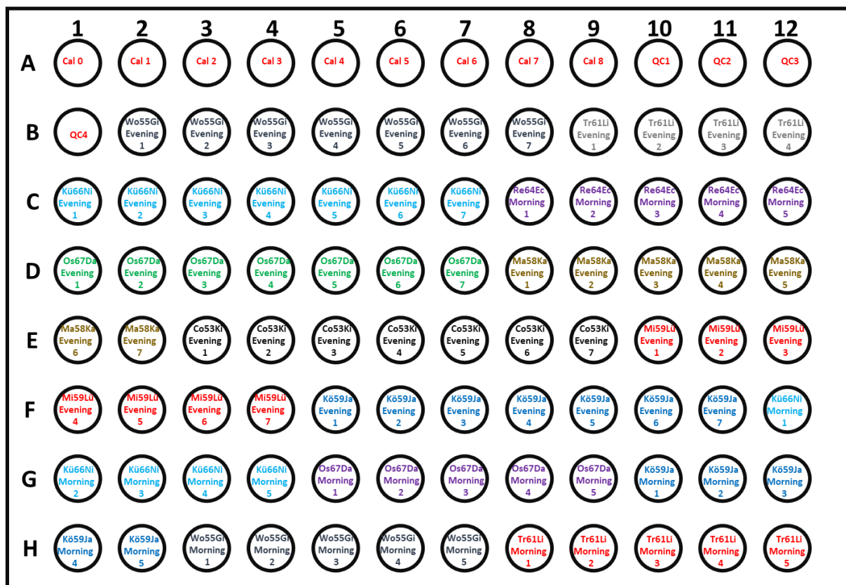
Fig. S2 Scheme of a 96 Well Plate template example for sample preparation. Cal and QC represent here calibrants and quality control samples, respectively and the rest are patient samples that are encoded.
