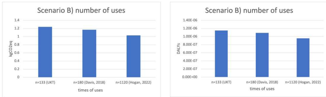
Figure 22: Environmental and Health impact scenario B) number of uses until end of life (EOL): Kilogram CO 2 equivalents & DALYs resulting from n=133 (University Hospital Tübingen), n=180 (Davis 2018) and n=1120 (Hogan 2022) times of uses.
