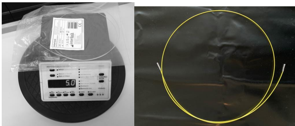
Figure 13: Example reprocessing reusable fURS: brush. Weight of brush without cover: app. 1g; brush in plastic cover: 5g, plastic cover single: 3.5g -> weight brush: app. 1.5g. Pictures taken by Marlene Thöne at the UKT.
