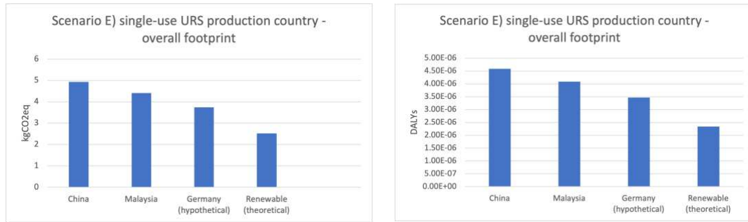
Figure 25: Environmental and Health impact scenario E) kg CO 2 eq & DALYs resulting for production process of single-use fURS in China vs. kg CO 2 eq resulting for production process in Malaysia, Germany (hypothetically) and with renewable energy mix (theoretically).
