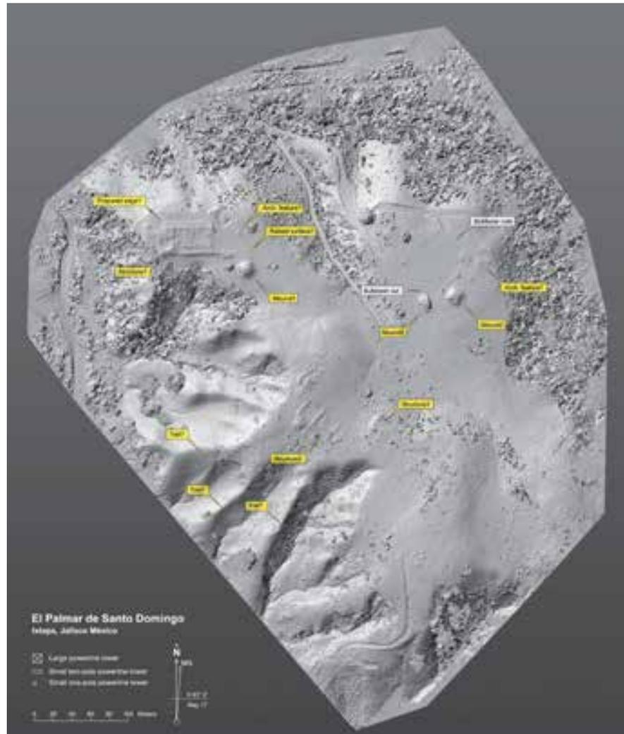
**Figure 10.** Annotated map of the Santo Domingo site with a DSM generated from Agisoft Photoscan as the base layer. Note the visible bulldozer tracks and damaged mound in the northeast portion of the site which were not visible in the orthomosaic.
