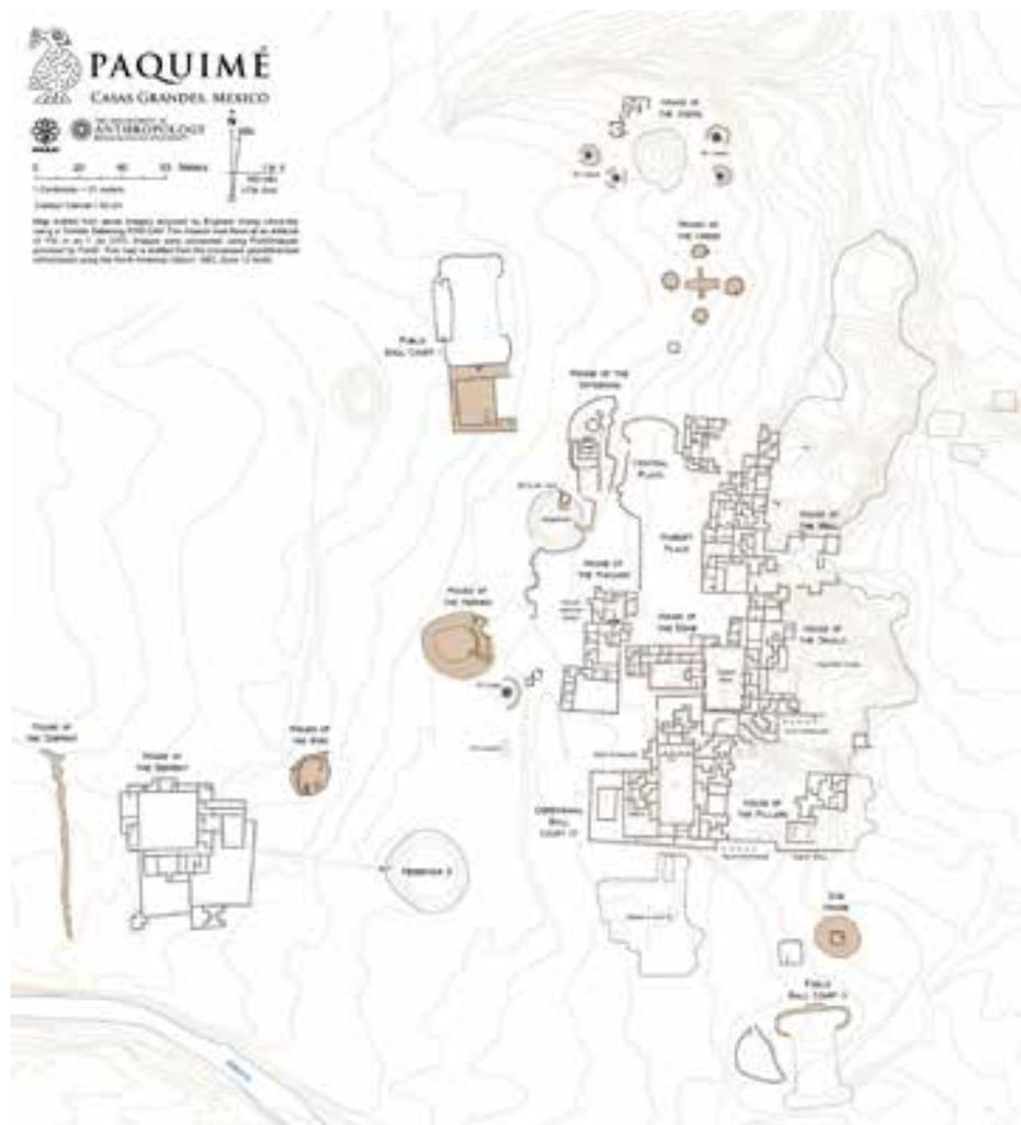
**Figure 7.** Map drafted in Adobe Illustrator using the Avenza MAPublisher plug-in. Contours were generated from a digital elevation model produced from the orthomosaic created in Pix4Dmapper. Architectural features were drawn directly from the orthomosaic.
