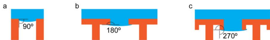
Figure S10. The edge angle of different fibrillar structures: a) simple pillars, b) T-shaped fiber structures, and c) double re-entrant fiber structures.
