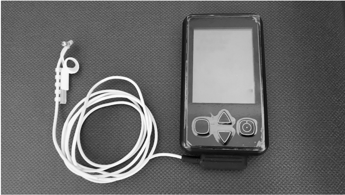
Figure 1: NEMOS Vagus nerve stimulation device that we used for transcutaneous auricular vagus nerve stimulation.
