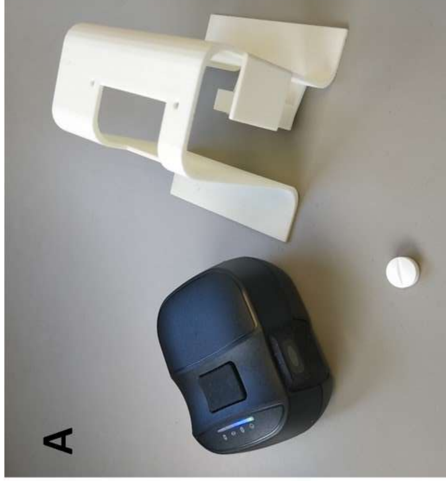
Supplementary Figure S1: (A) The NIR-S-G1 spectrometer, the 3D-printed device holder (designed by LuxFlux GmbH, Reutlingen, Germany), and a pharmaceutical tablet. (B) Assembly for spectra acquisition. The dice is included to illustrate the size of the device. (Photo: Gesa Gnegel, Tübingen University)
