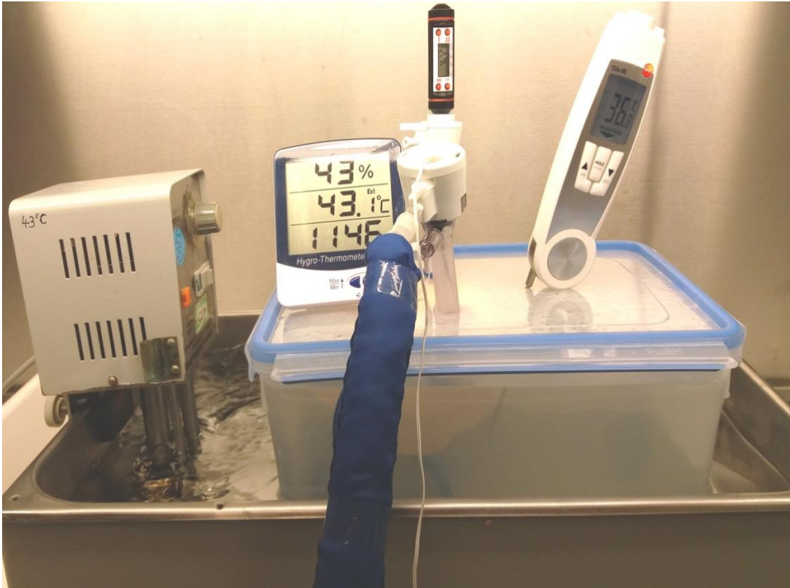
Figure 4: View of the experimental setting using the IBUB ex-vivo model. The IBUB is placed into a closed plastic container, which is immersed into a water bath kept at a constant temperature of 37 °C. Then, the IBUB is heated up with warm-humid CO 2 up (heated inflow tube, blue) until a temperature range between 41 °C – 43 °C is reached. The system is then ready for the heated chemotherapy application.
