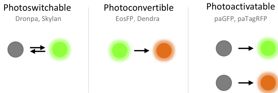
Figure 1-3: Overview of different types of photoactive fluorescing proteins used in super-resolution fluorescence microscopy. Grey circles indicate fluorescing proteins in a non-emitting fluorescent off state. Green and red circles represent fluorophores emitting respectively colored light.
