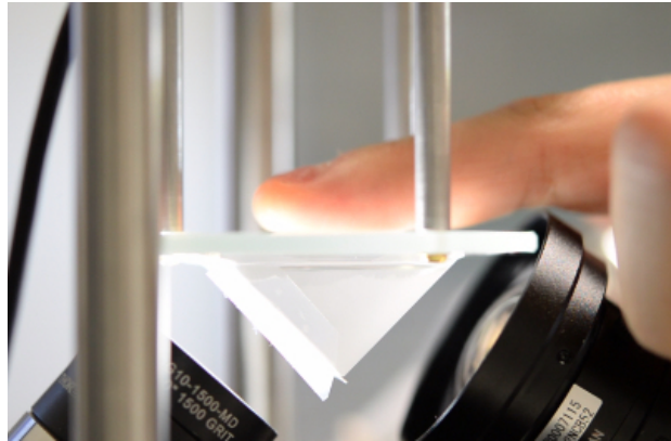
Figure 2.1: A soft finger's contact area develops in various ways depending on its material properties and how it is pressed into the surface (Photo by Nam and Kuchenbecker / CC BY).
