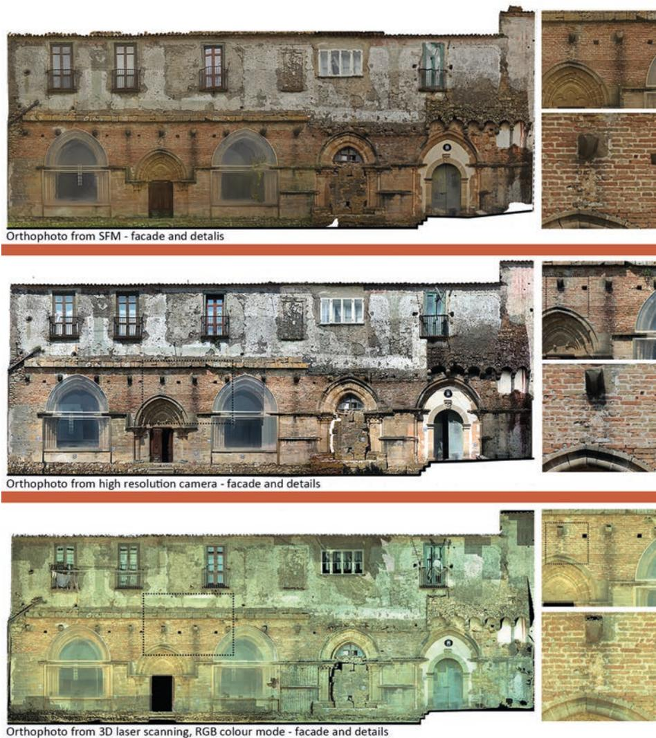
**Figure 9.** Orthophoto of the façade obtained through three different methodologies: High Resolution camera, Structure from Motion and Image Matching, Laser scanning-RGB mode. Comparison about RGB data.
