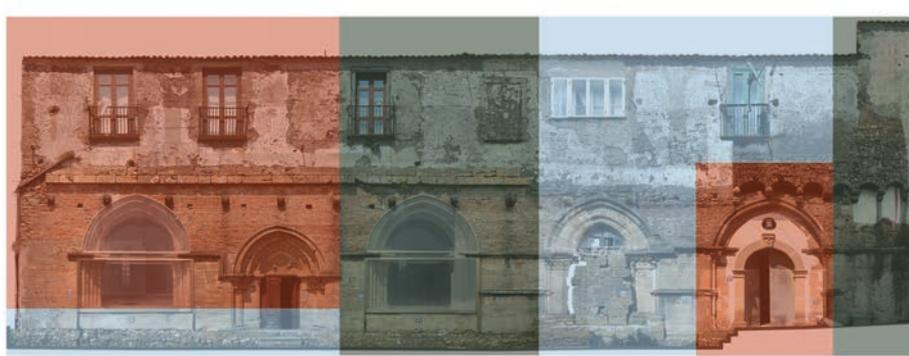
Figure 5. The construction of the orthophoto of the façade derived from high resolution camera.
