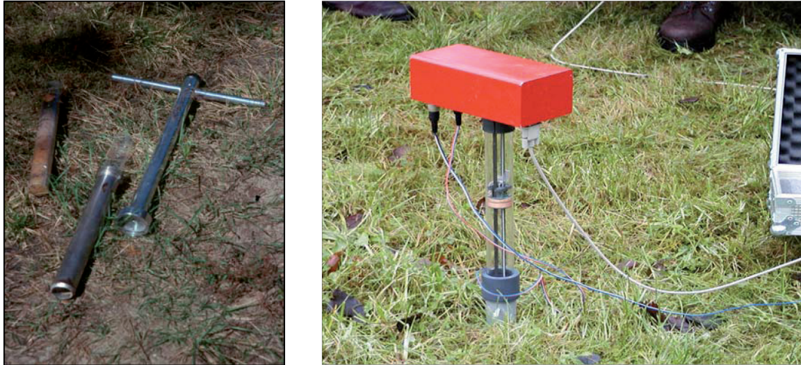
Fig. 2 Stainless-steel soil corer (40 mm outer diameter) plus a soil core sample are shown in (a). In (b) the MS400 down-hole susceptibility meter (ZH instruments) is presented.
