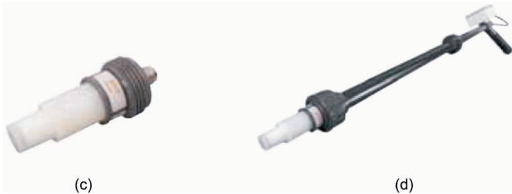
Fig. 1 Bartington MS2 susceptibility meter (a), MS2D-sensor (b), MS2F-sensor (c) and probe handle for MS2D and MS2F sensors.
