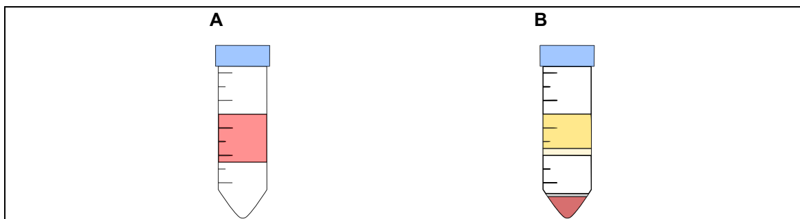
Figure 7: Density gradient centrifugation modified according to [46, 68, 100]. A Whole blood layered onto a substrate of specific molecular weight: whole blood (light red) and substrate (white). B Separation of whole blood components following density gradient centrifugation: plasma and platelets (orange), PBMC (yellow), substrate (white), granulocytes (grey) and erythrocytes (dark red).
