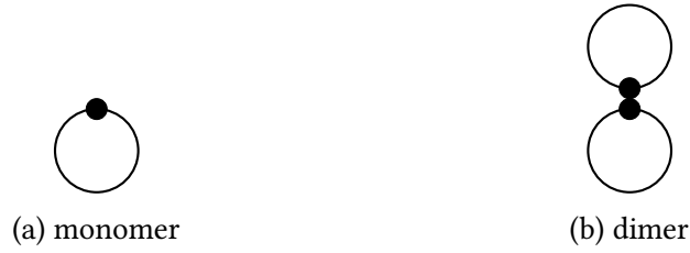
Figure 4.1: Monomers and dimers from Wertheim's original formulation. The circles represent colloids with a single bonding site.
